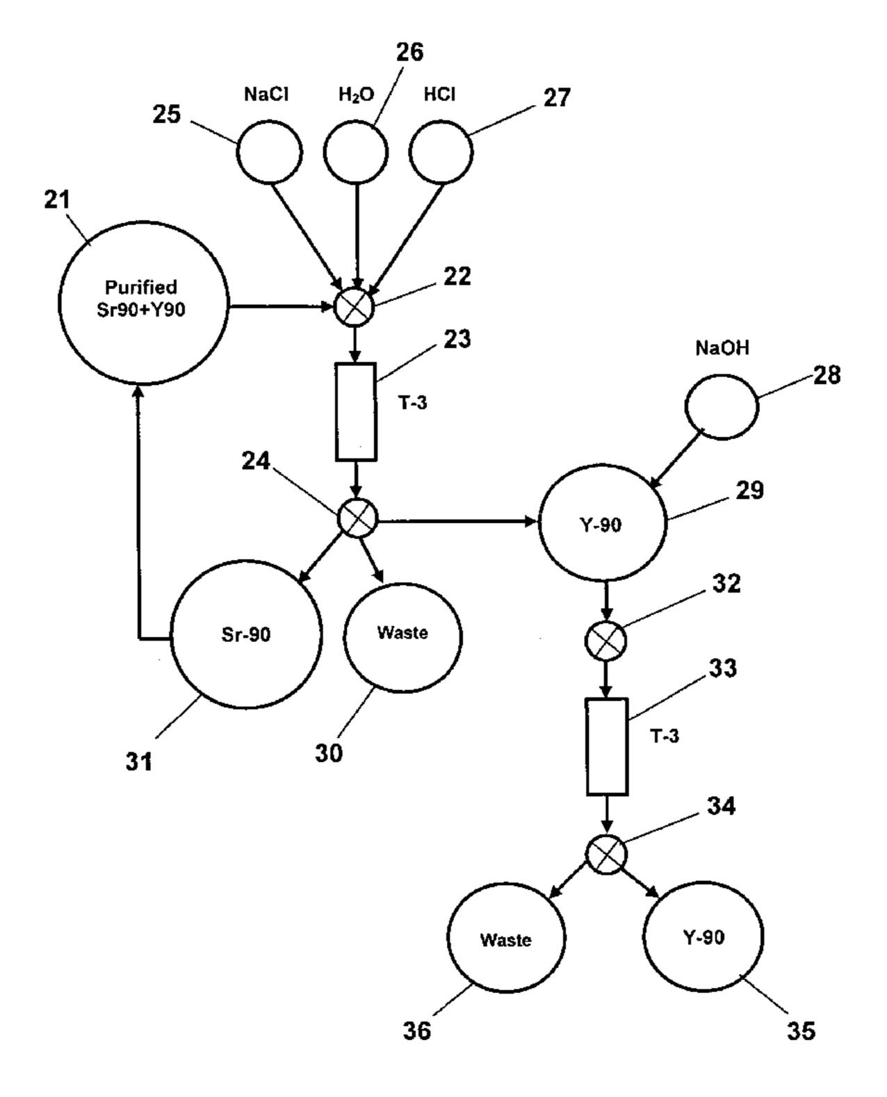
Fig. 1 Stage 1: Purification of Sr-90 Stock Solution
