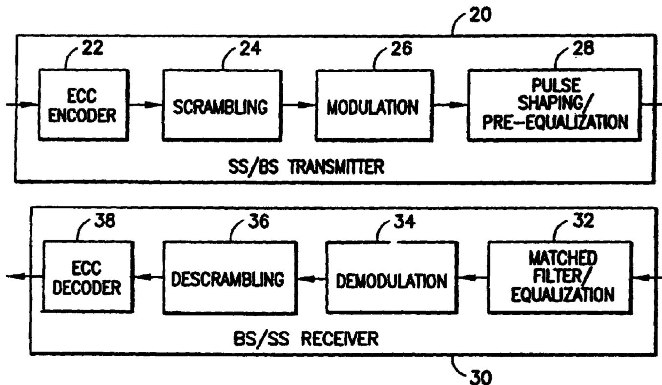
**FIG 2** PHY REFERENCE MODEL SHOWING DATA FLOW
