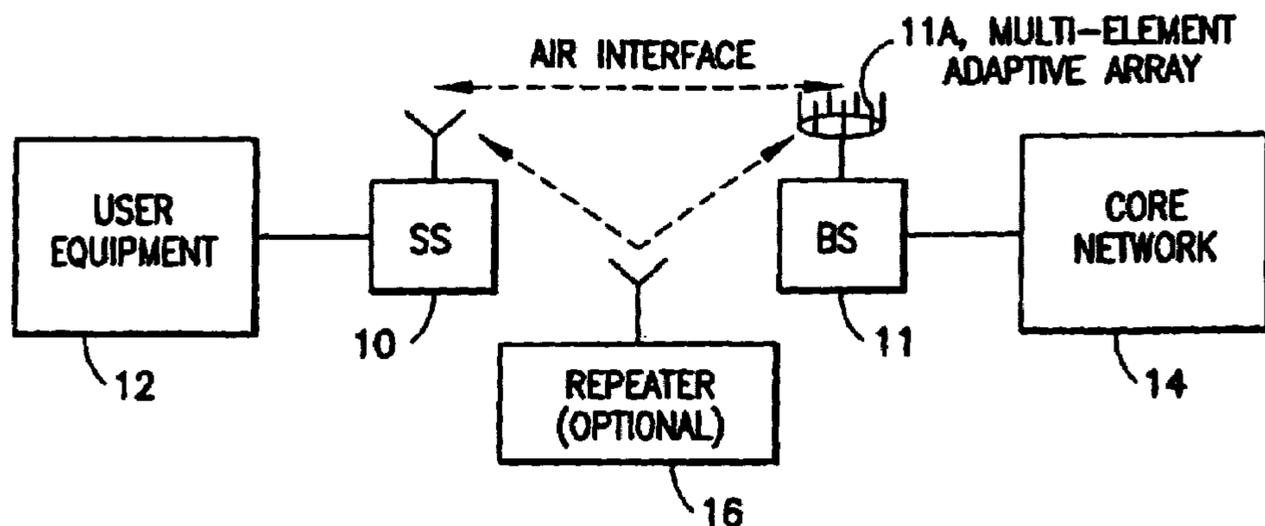
**FIG. 1** WIRELESS ACCESS REFERENCE MODEL
