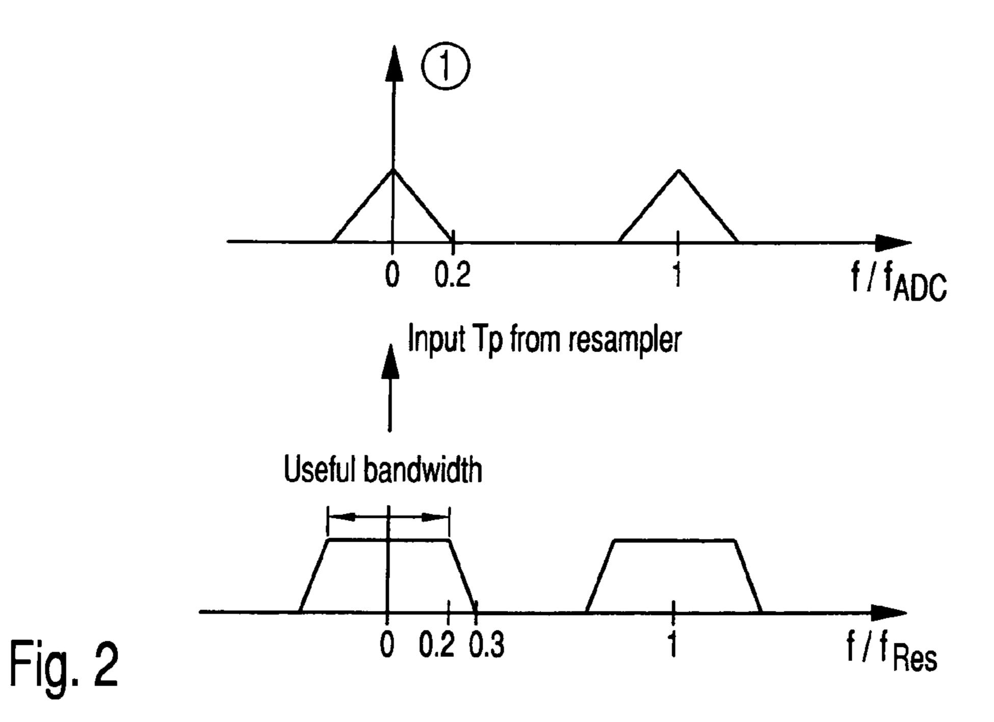
f/f<sub>ADC</sub> 0.2 f/f<sub>Res</sub> 0.2 Input Tp from resampler Useful bandwidth 0 0.2 0.3
