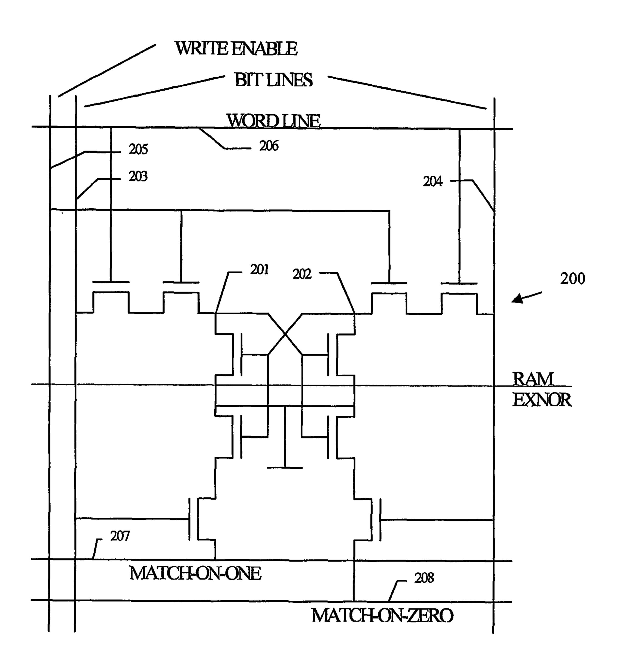
Figure 3 ASP word-organised 10-transistor CAM cell
