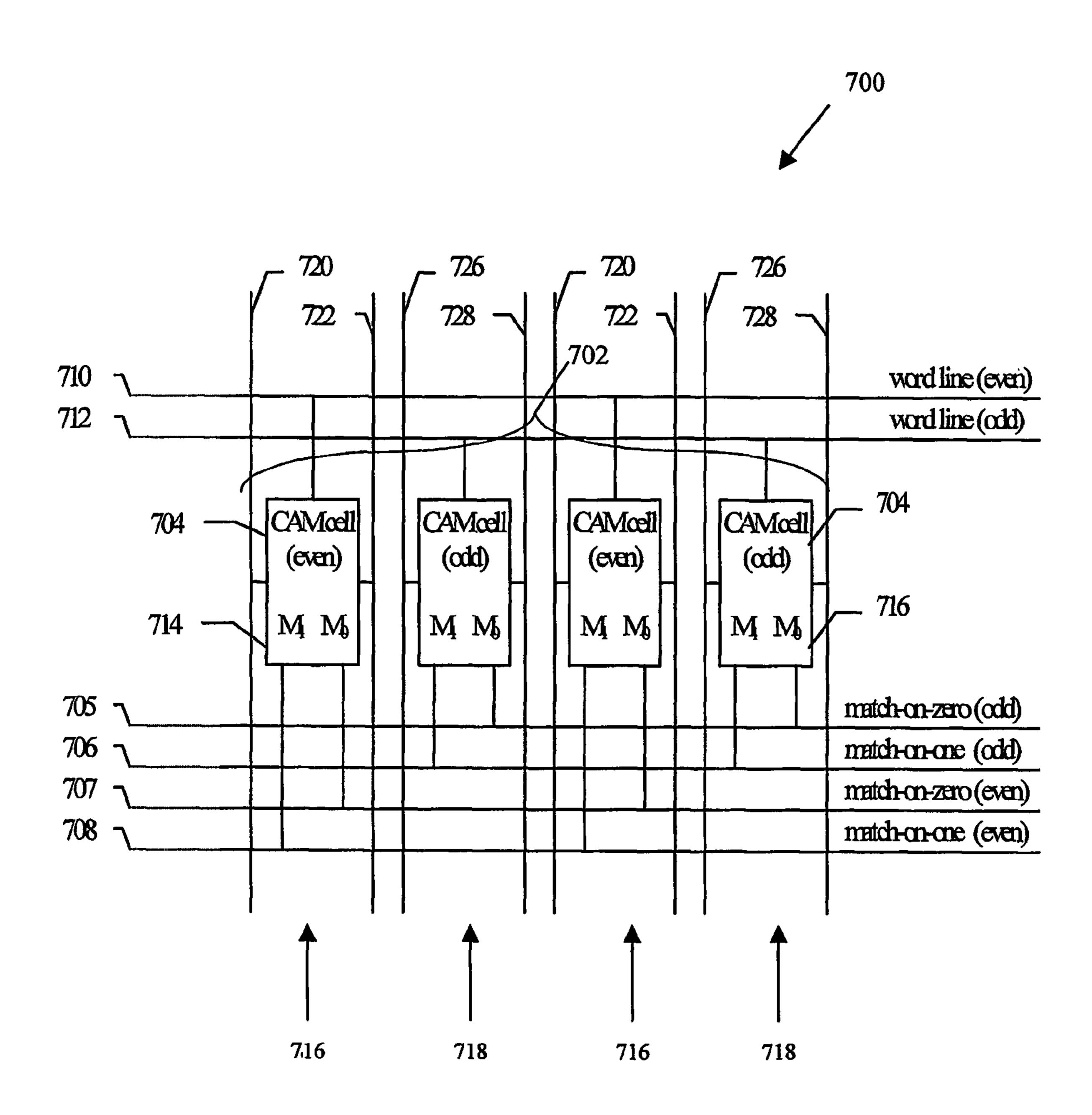
Figure 8 Interleaved memory bits for enhanced numeric capability, improved speed and reduced power
