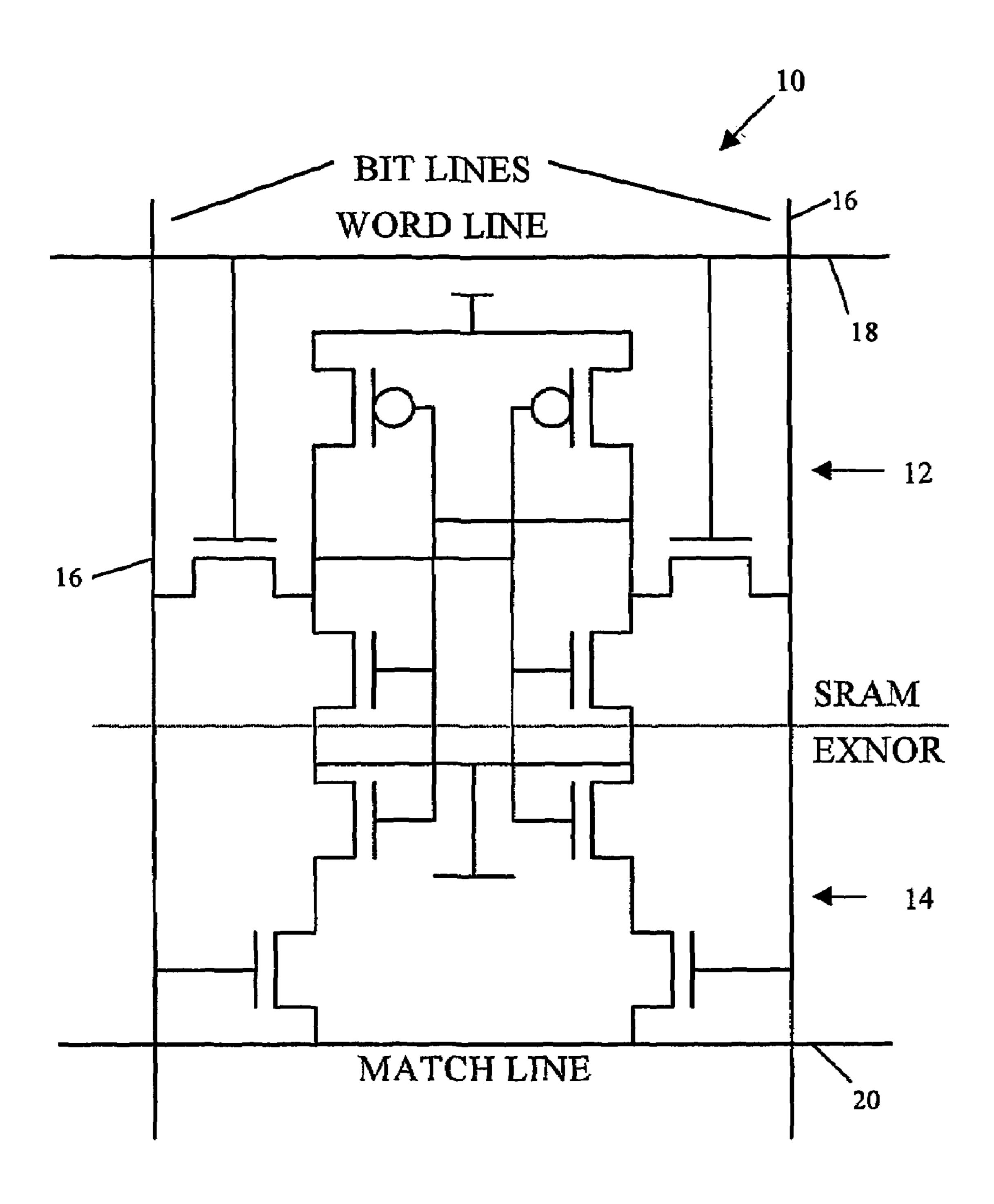
Figure 1 Prior-art SRAM-based CAM cell
