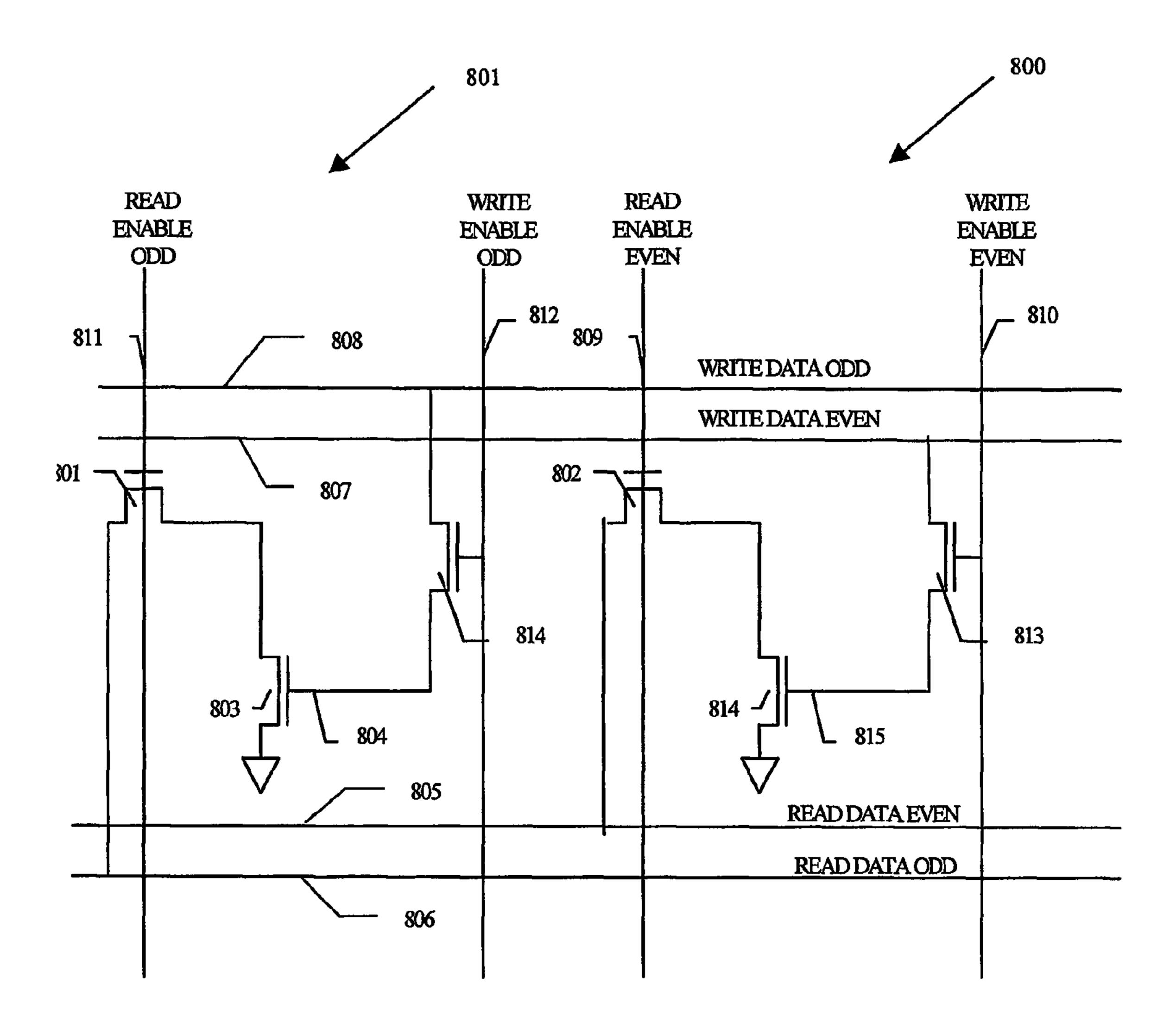
Figure 9 Extended-memory organisation for two-bits-at-a-time operation
