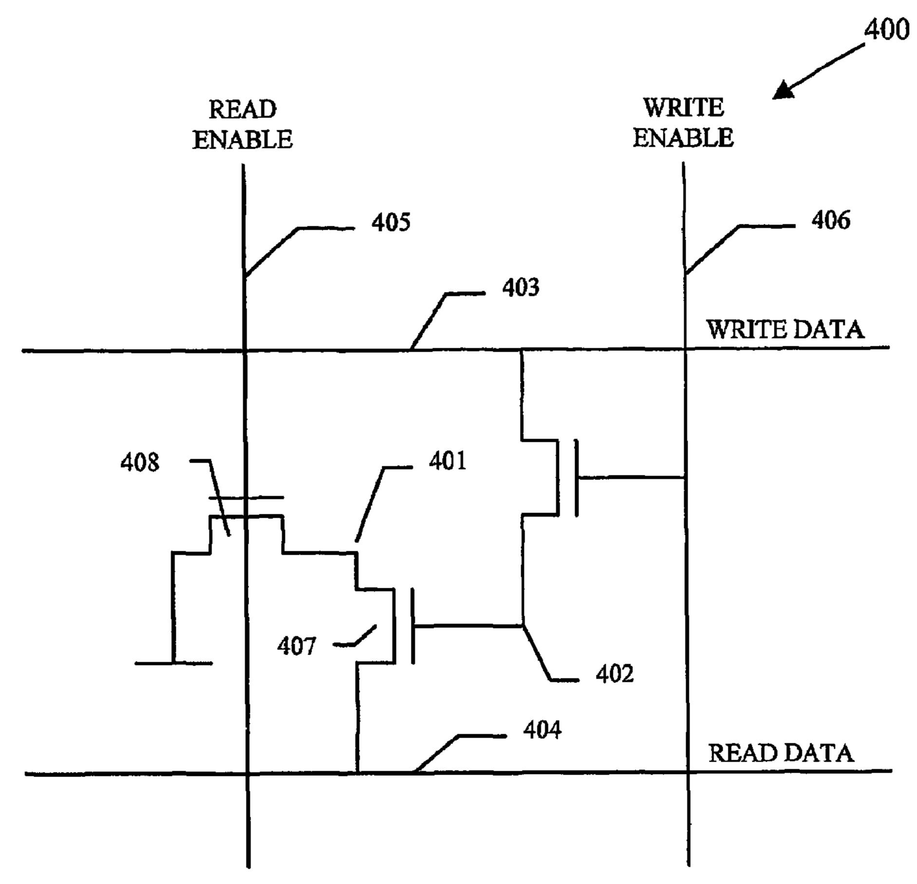
Figure 5 3-transistor extended memory cell
