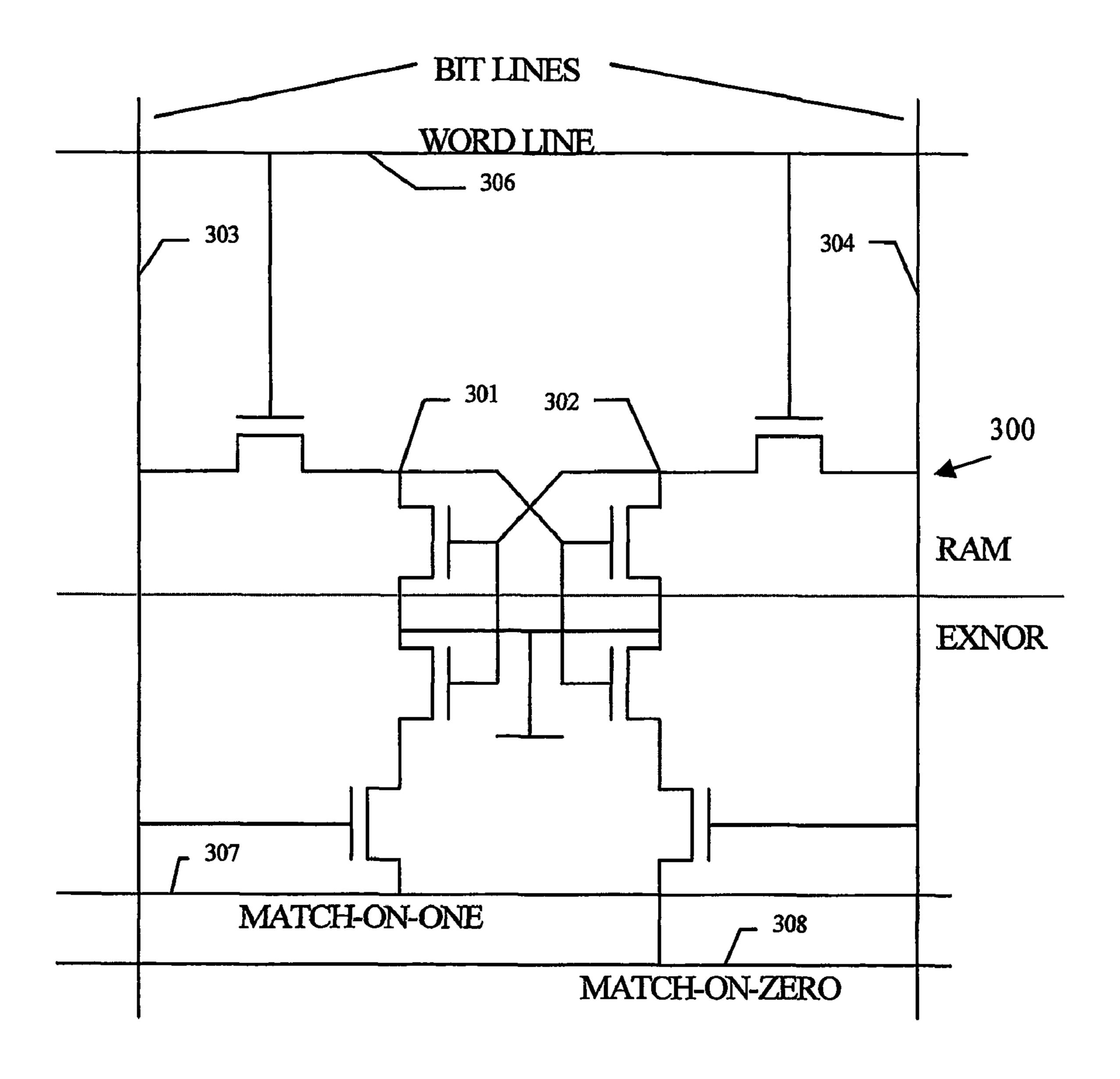
Figure 4 Alternative non-explicit mask CAM cell
