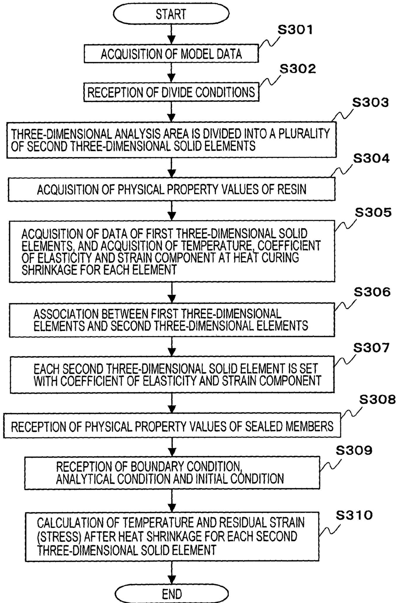
STEP S3 (CALCULATION OF RESIDUAL STRAIN (STRESS))
