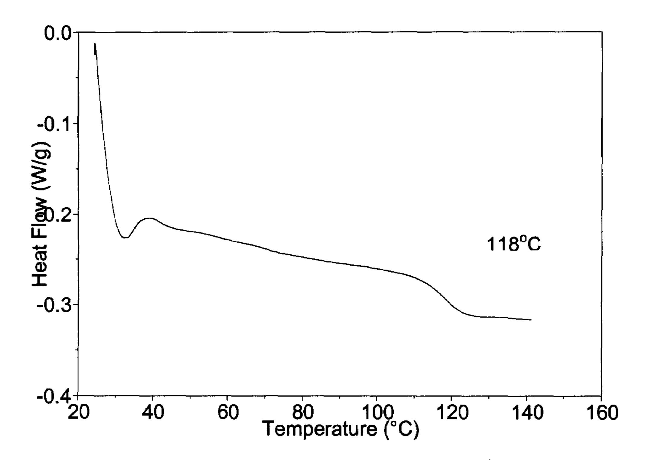
DSC: Heat Polymerized PMMA/SWNT Composite
