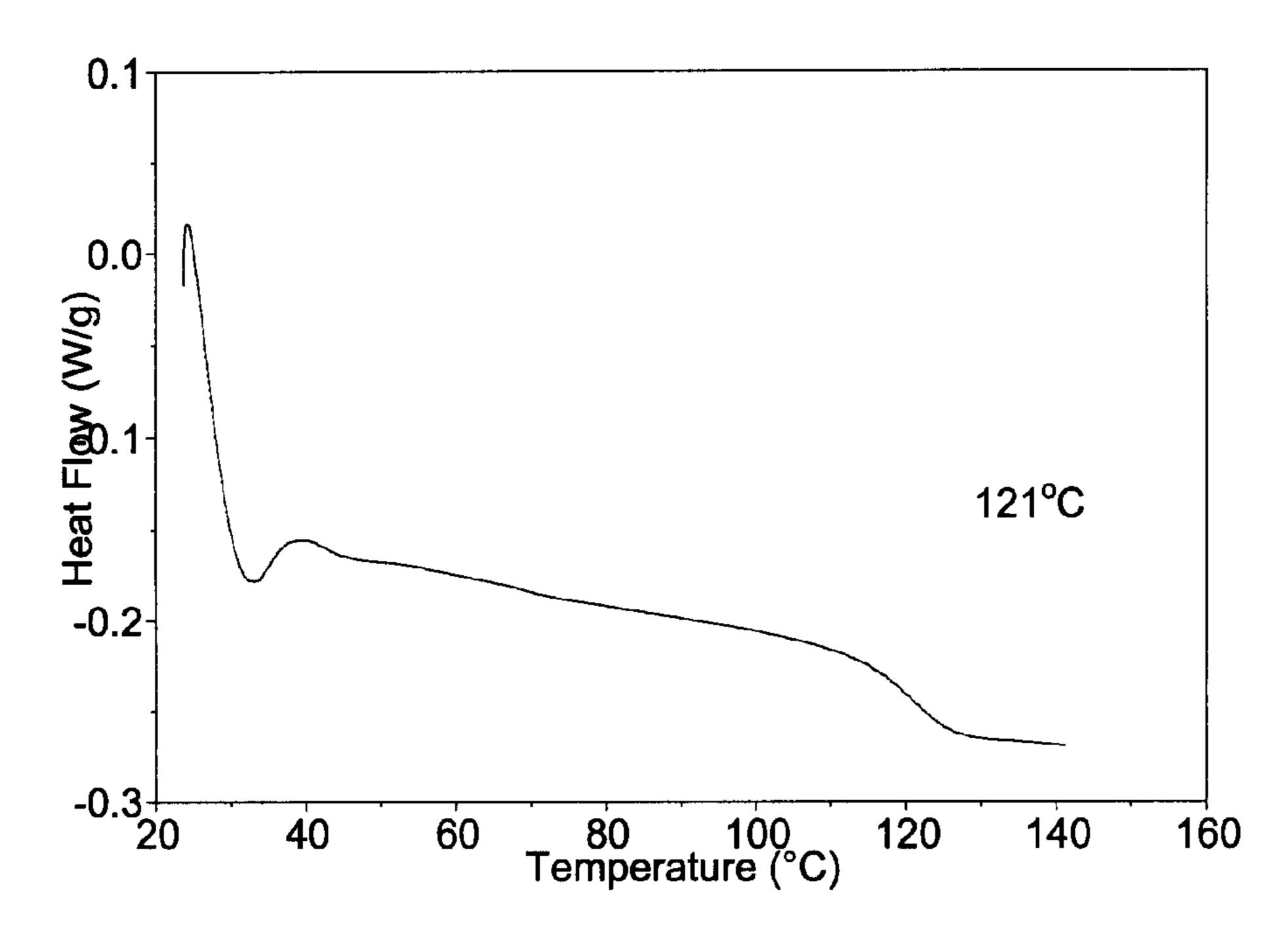
DSC: lonizing (gamma) Radiation polymerized neat PMMA
