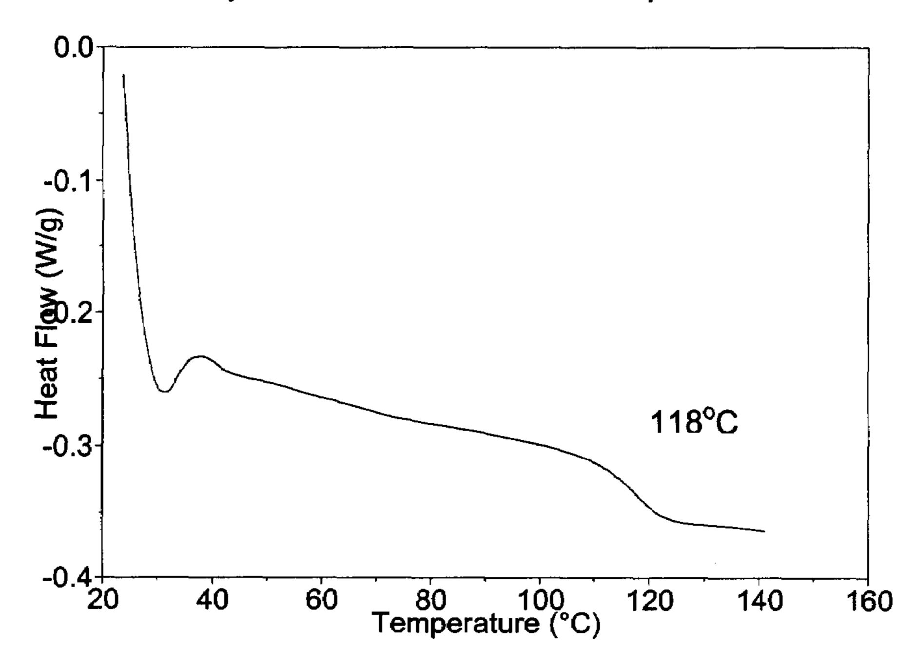
FIG 9 DSC: lonizing (gamma) Radiation Polymerized PMMA/SWNT Composite
