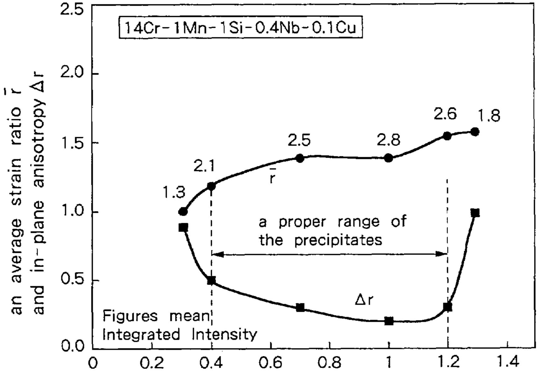
a total ratio (mass %) of precipitates of  $0.5\,\mu m$  or less in particle size in a steel matrix before finish-annealed
