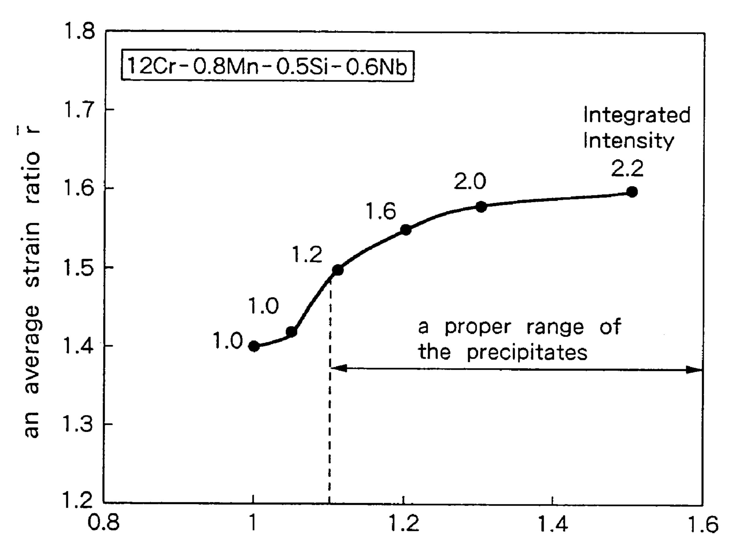
a total ratio (mass %) of precipitates of 2 µm or less in particle size in a steel matrix before finish-annealed
