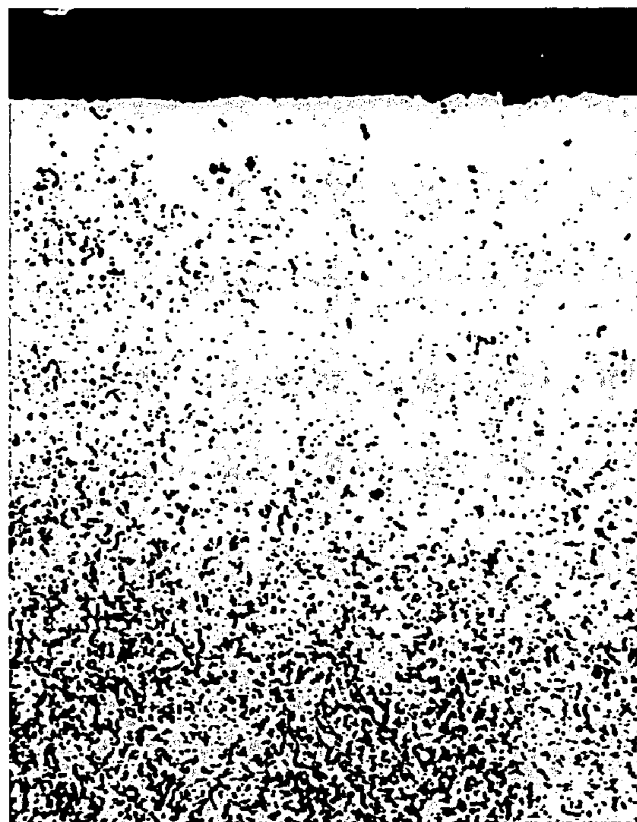
AFTER SPHERODIZING ANNEALING PATTERN 1 SURFACE LAYER X 100
