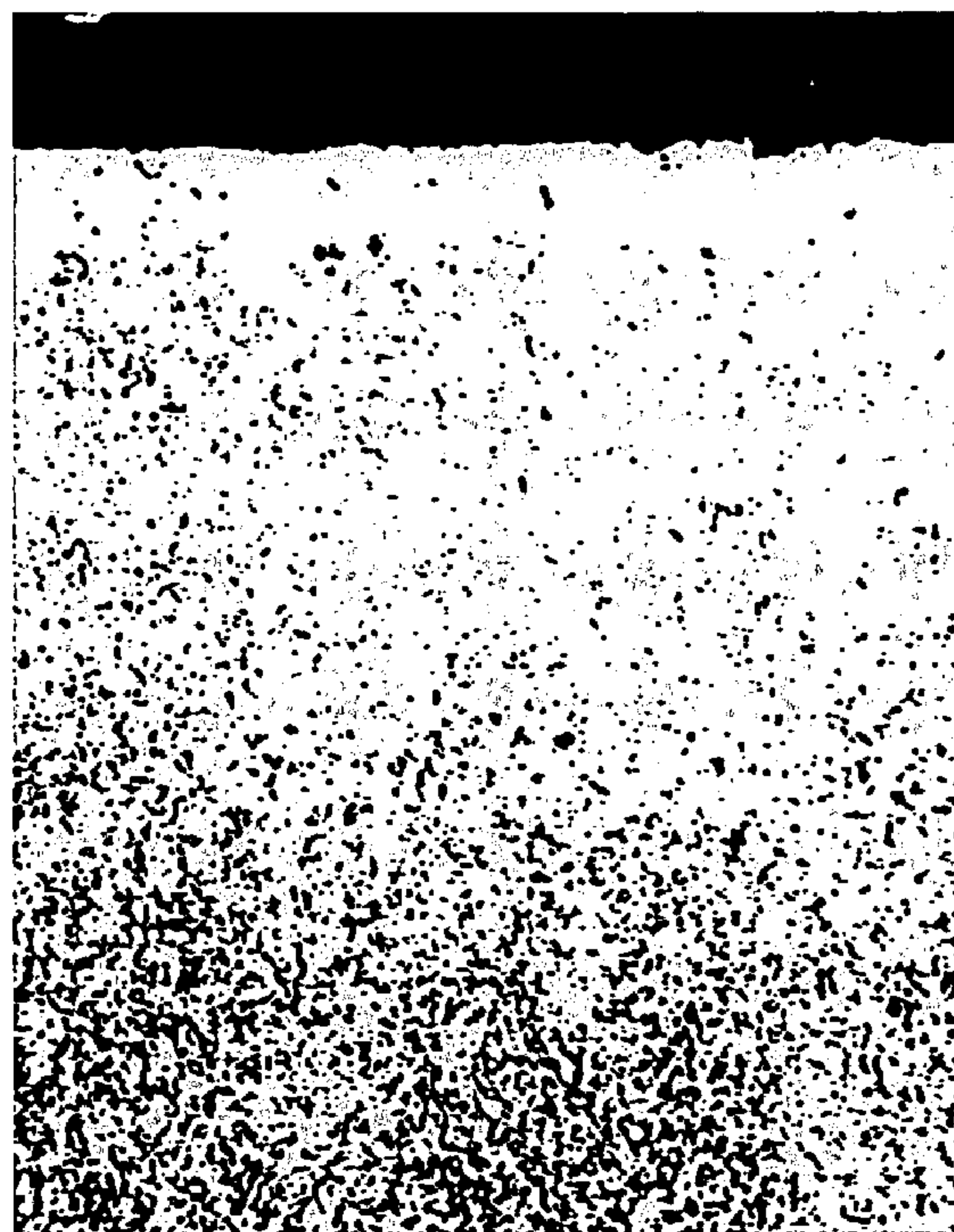
AFTER SPHERODIZING ANNEALING PATTERN 1 SURFACE LAYER X 100
