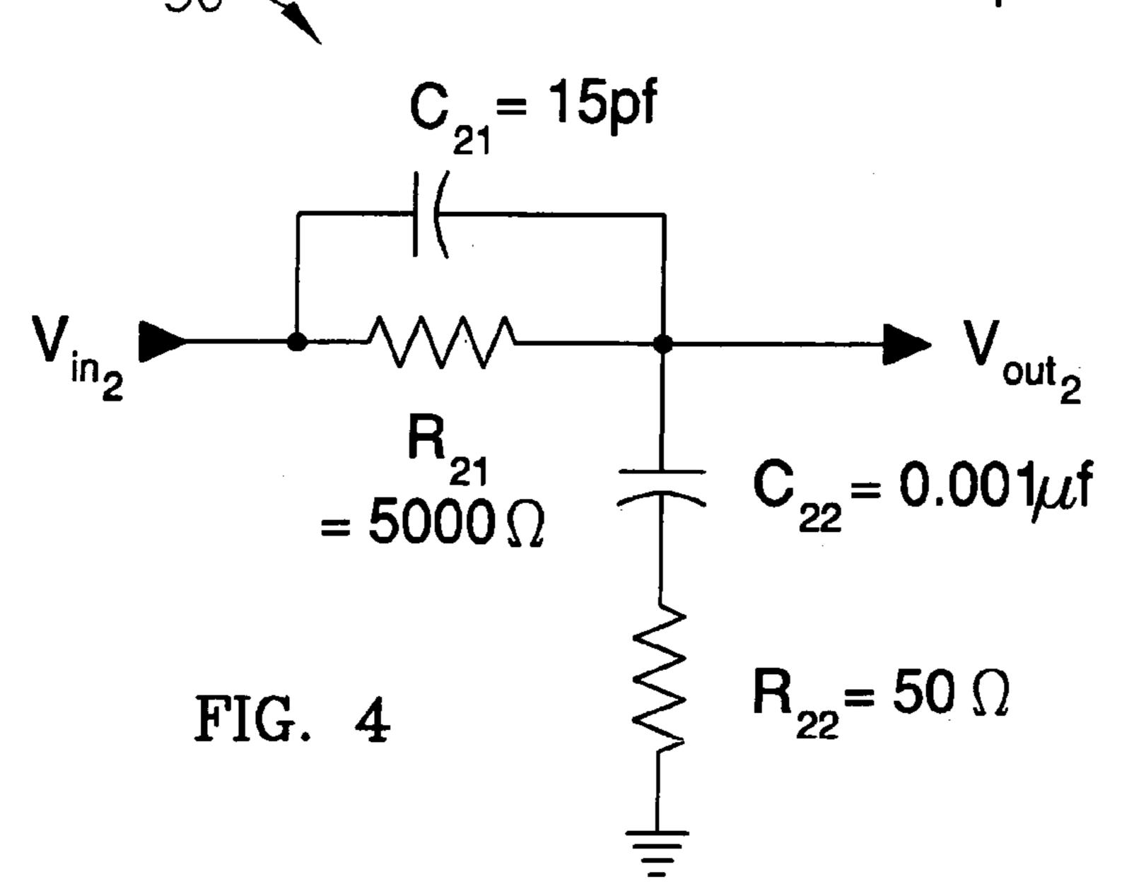
$$\frac{V_{\text{out}_2}}{V_{\text{in}_2}} = \frac{(R_{21}C_{21}s + 1)(R_{22}C_{22}s + 1)}{R_{21}C_{21}R_{22}C_{22}s^2 + (R_{21}C_{21} + R_{22}C_{22} + R_{21}C_{22})s + 1}$$
