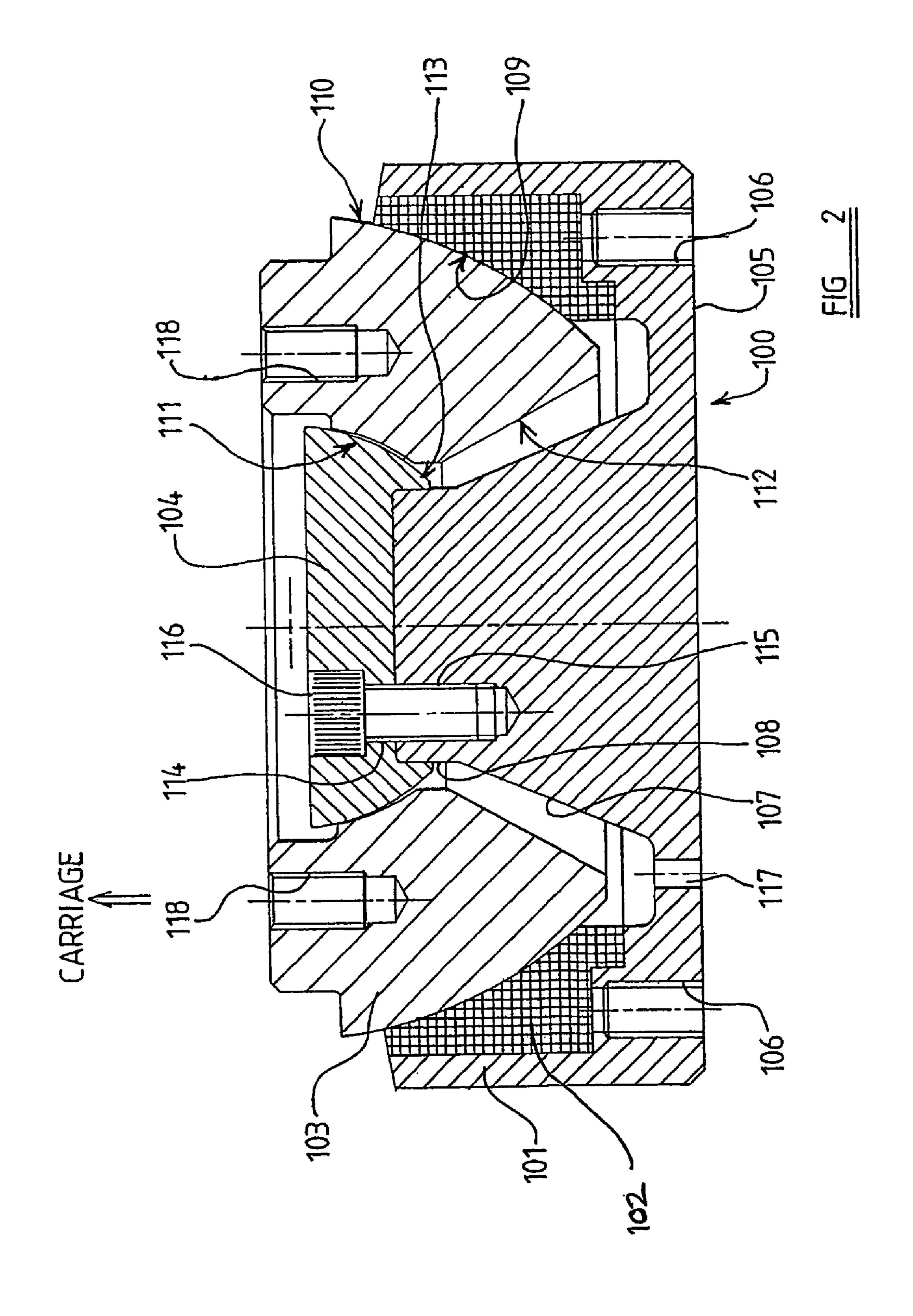
This invention relates to a thrust bearing and more particularly to a thrust bearing for use as a tram and light rail coupling bearing.
