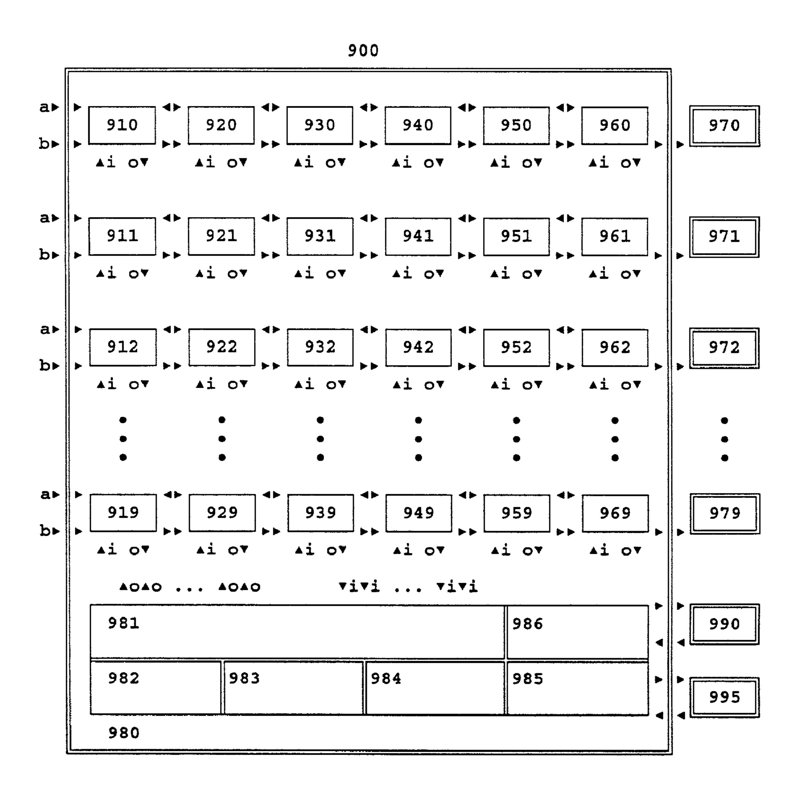
FIGURE 9B: SECOND SYSTEM DIAGRAM OF SETTOP BOX OR OTHER DEVICE
