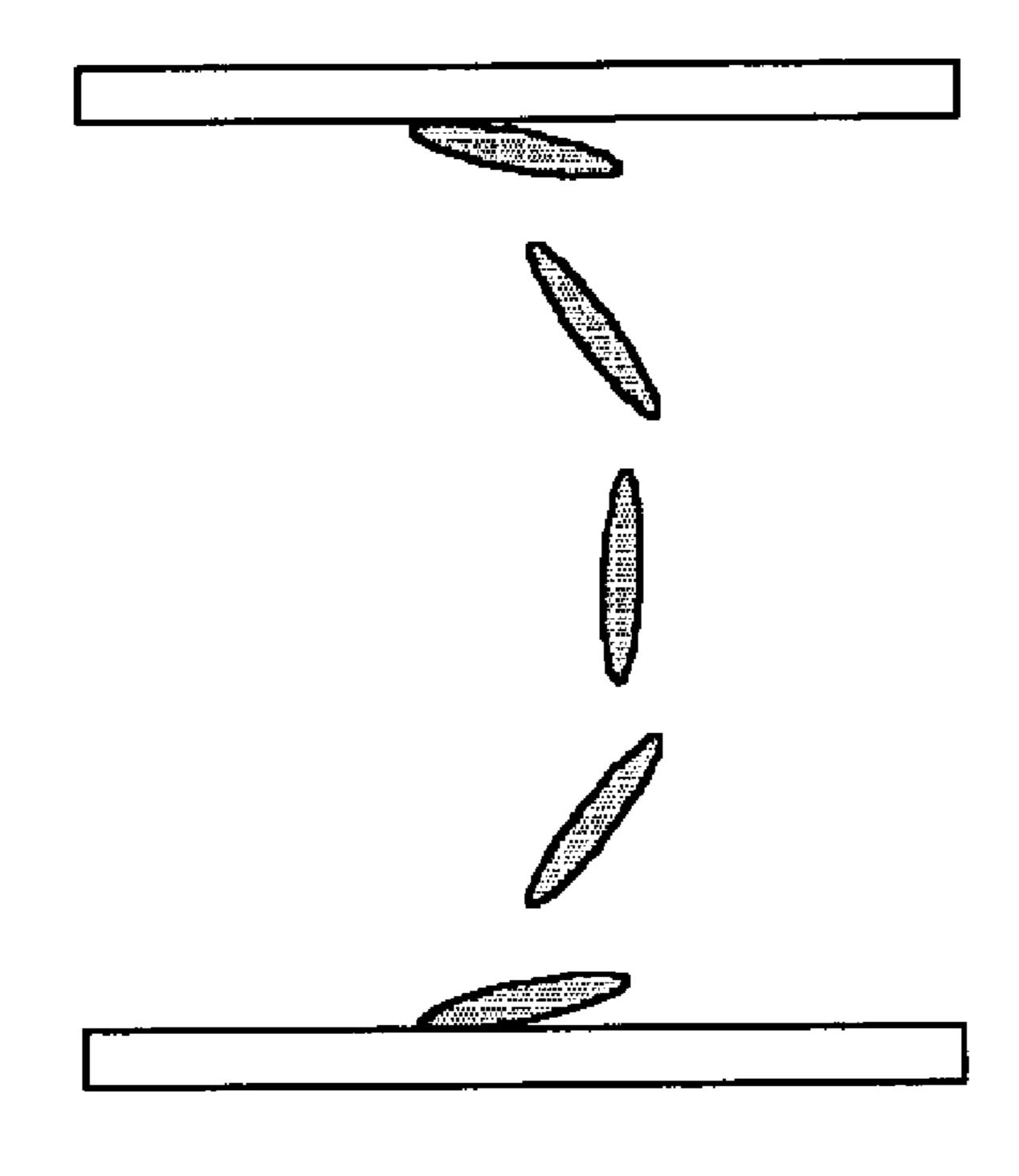
Bend state when a transition voltage is applied
