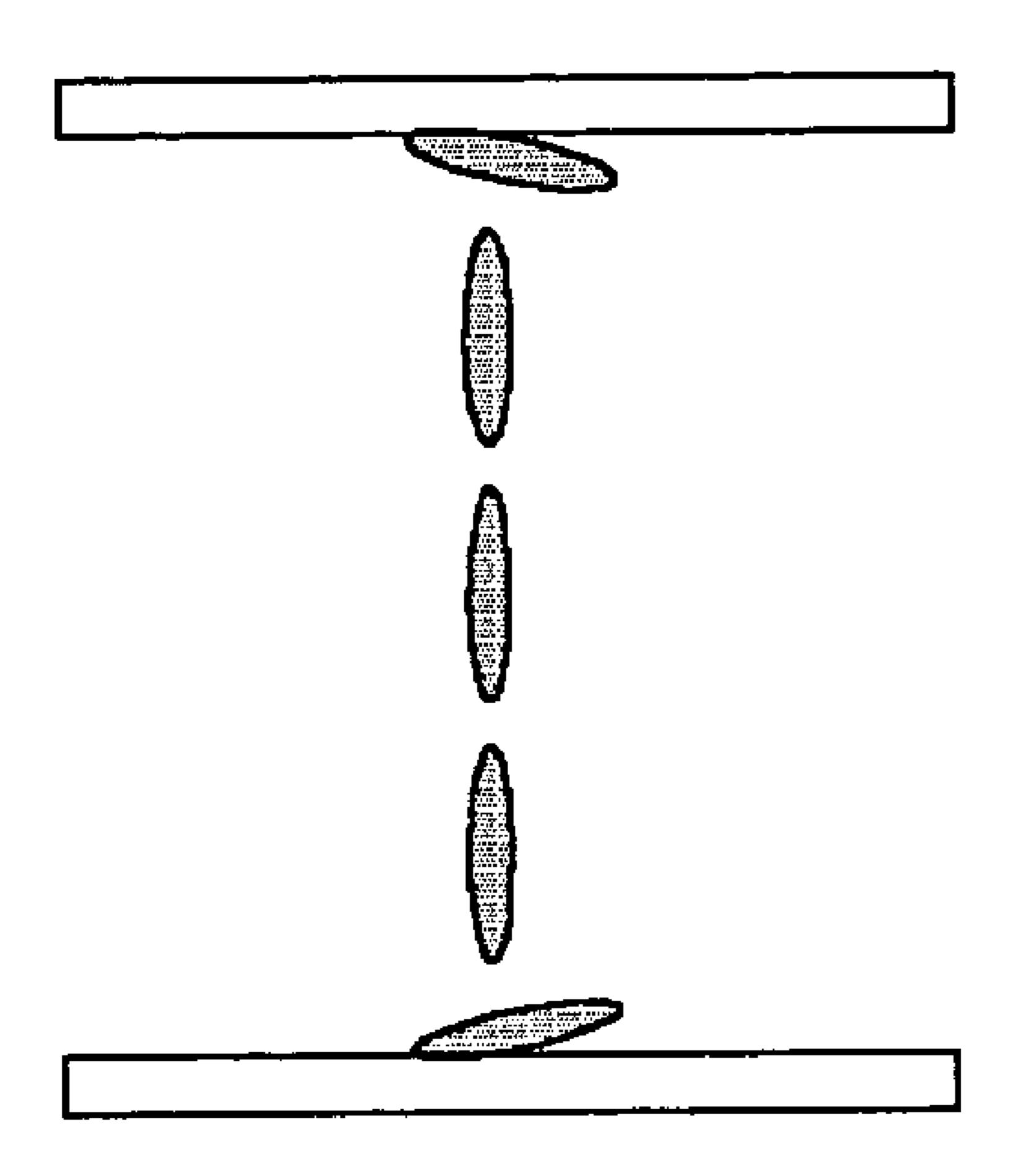
Vertically aligned when voltages are applied
