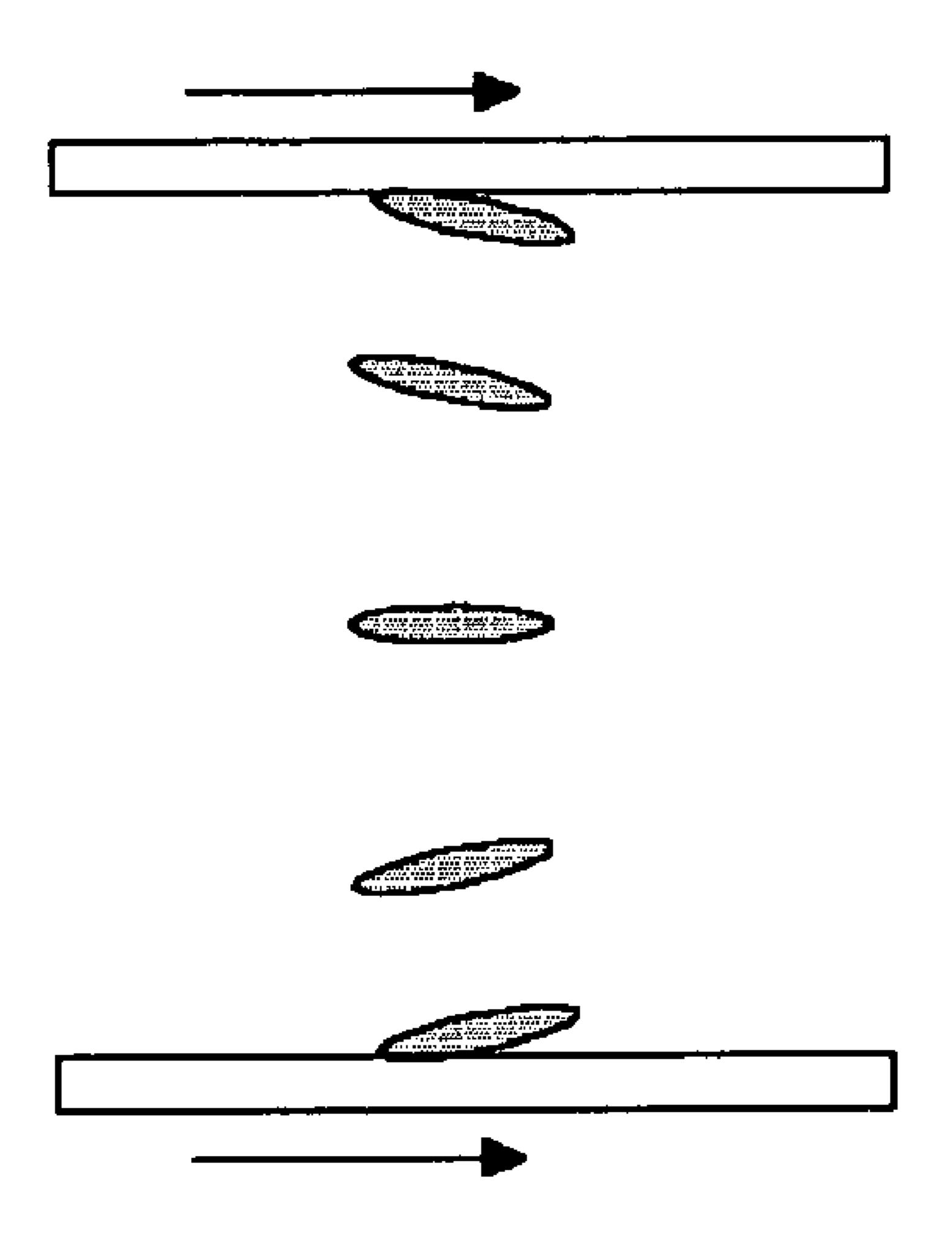
Splay state when a voltage is not applied
