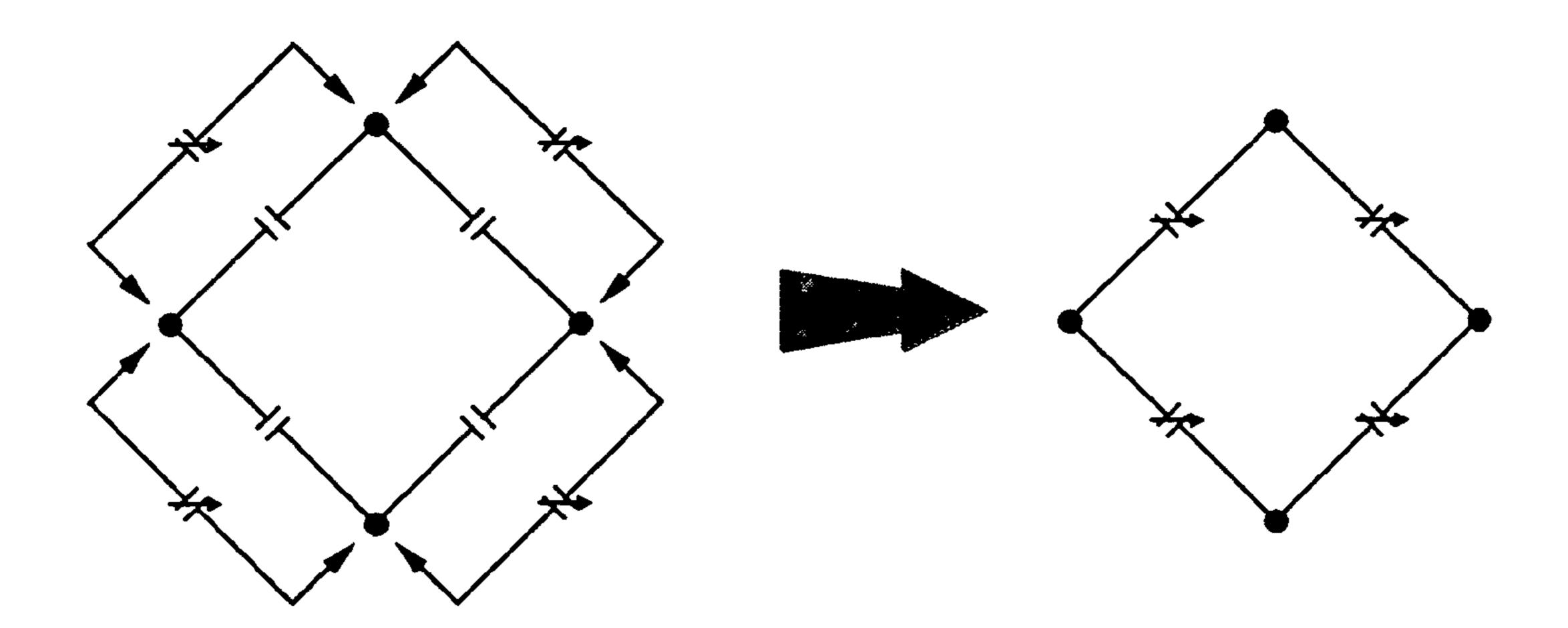
Insert variable capacitor between each Excite/detect electrode pair
