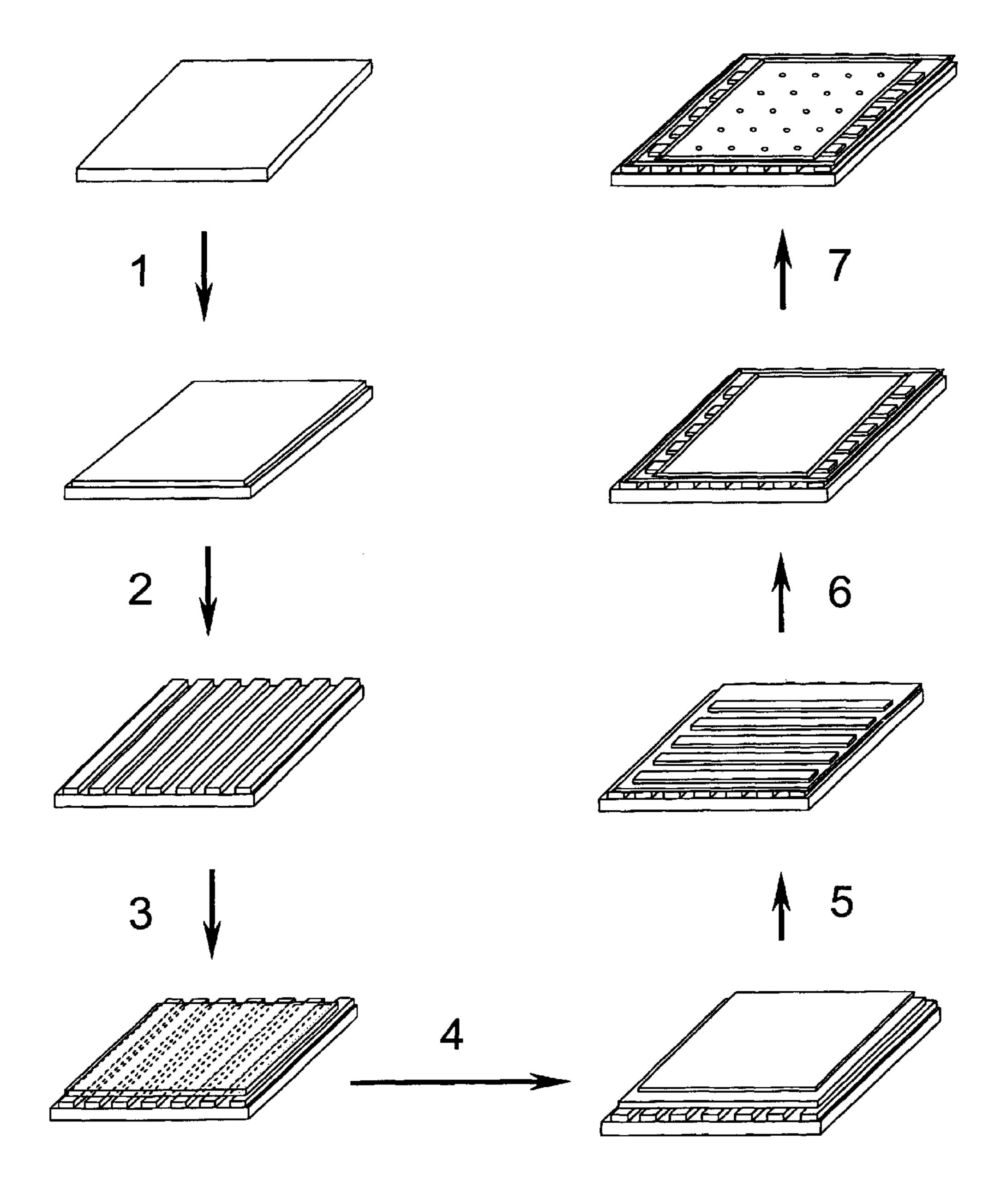
Fabrication procedures of molecular well-embedded architectures
