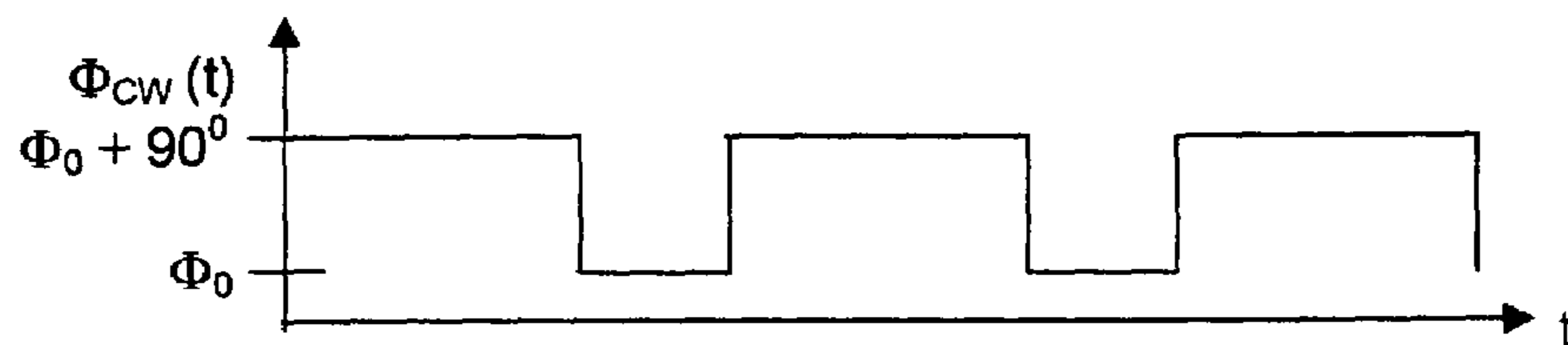
FIGURE 3 3-Point Modulation Waveform
