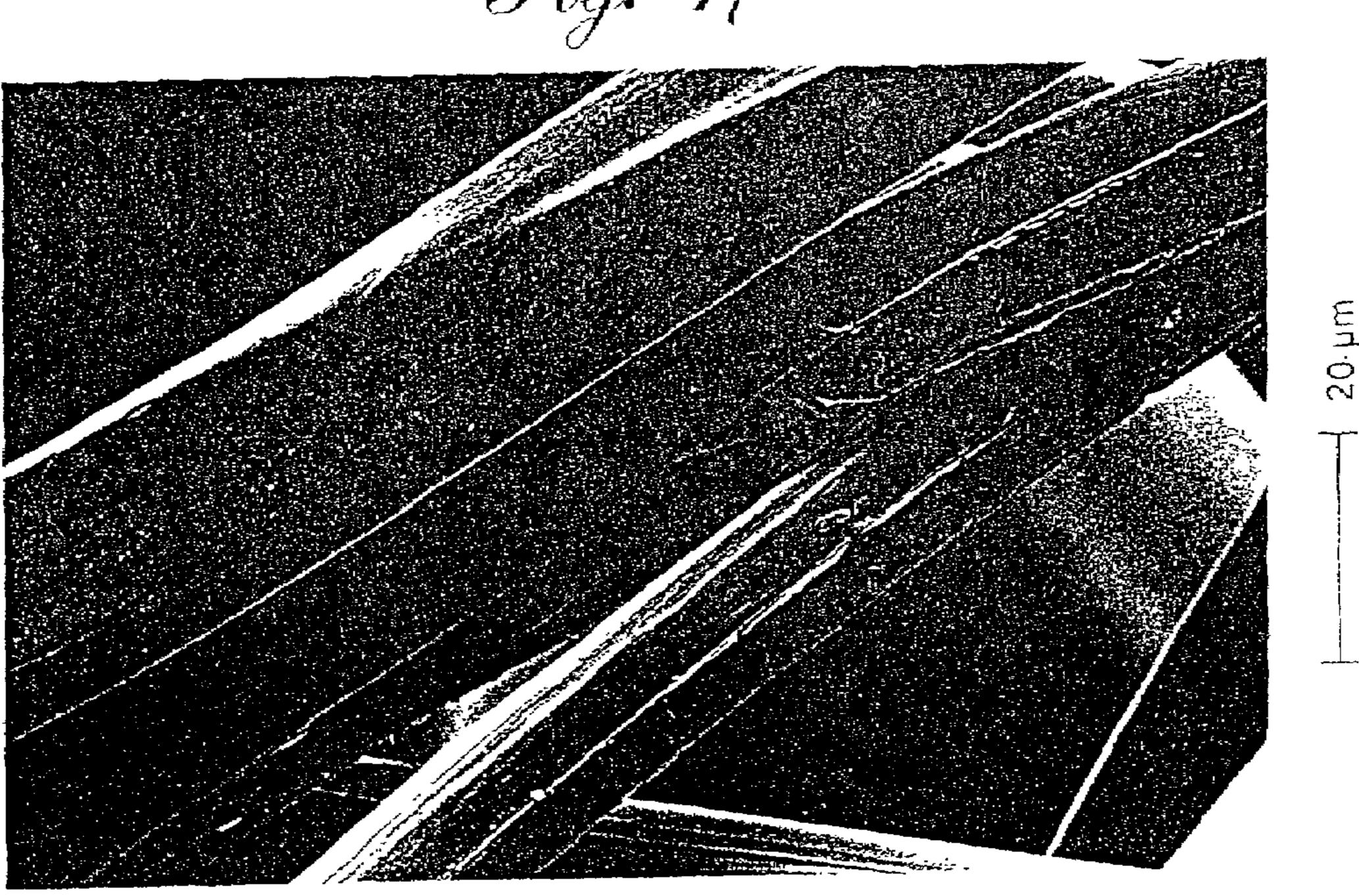
Abraded Melt Blown Fiber 2 - 1000X
