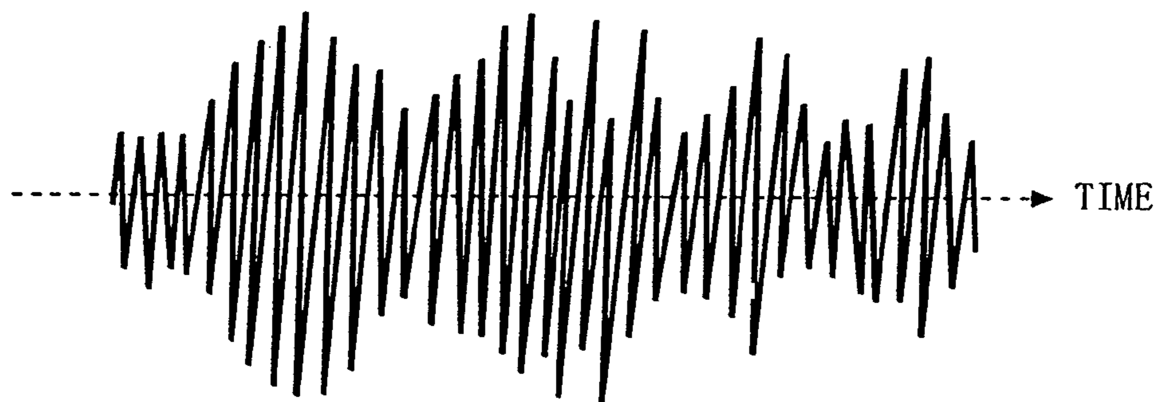
FREQUENCY-MULTIPLEXED SIGNAL WITH INSTANTANEOUS AMPLITUDE VARIATION SUPPRESSED
