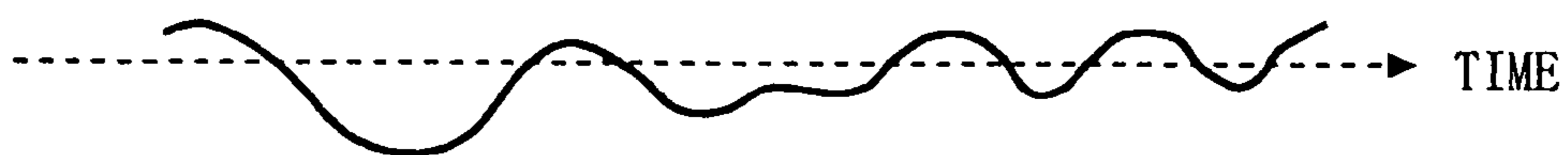
DETECTION SIGNAL DETECTING INSTANTANEOUS AMPLITUDE VARIATION OF FREQUENCY-MULTIPLEXED SIGNAL (AFTER PHASE ADJUSTMENT)
