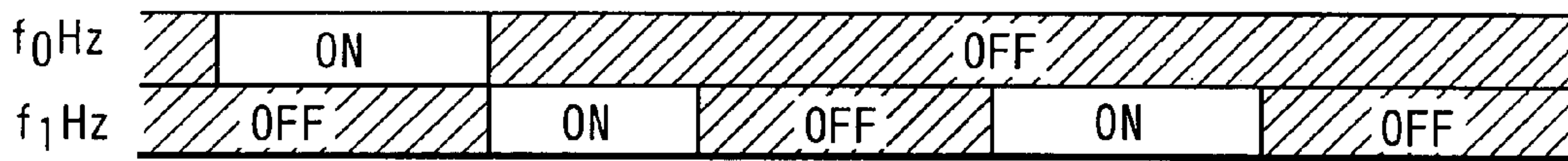
OPERATION EXAMPLE OF FILTER 0 (ON: PASS DATA OFF: INTERRUPT DATA)
