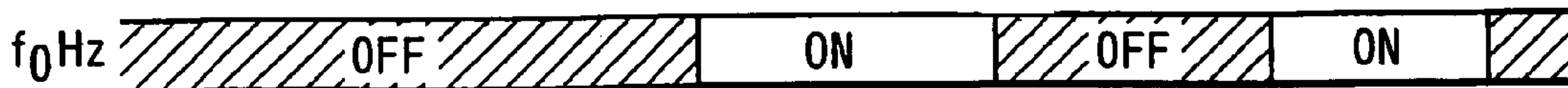
OPERATION EXAMPLE OF FILTER 1 (ON : PASS DATA OFF : INTERRUPT DATA)
