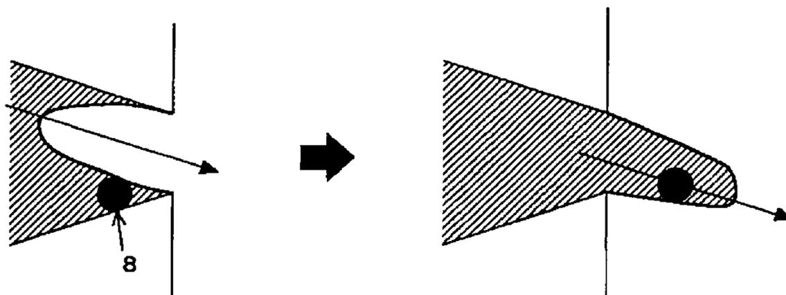
(b) In the case the meniscus is axially symmetric (the case that the nozzle diameter is large relatively to the particle diameter).
