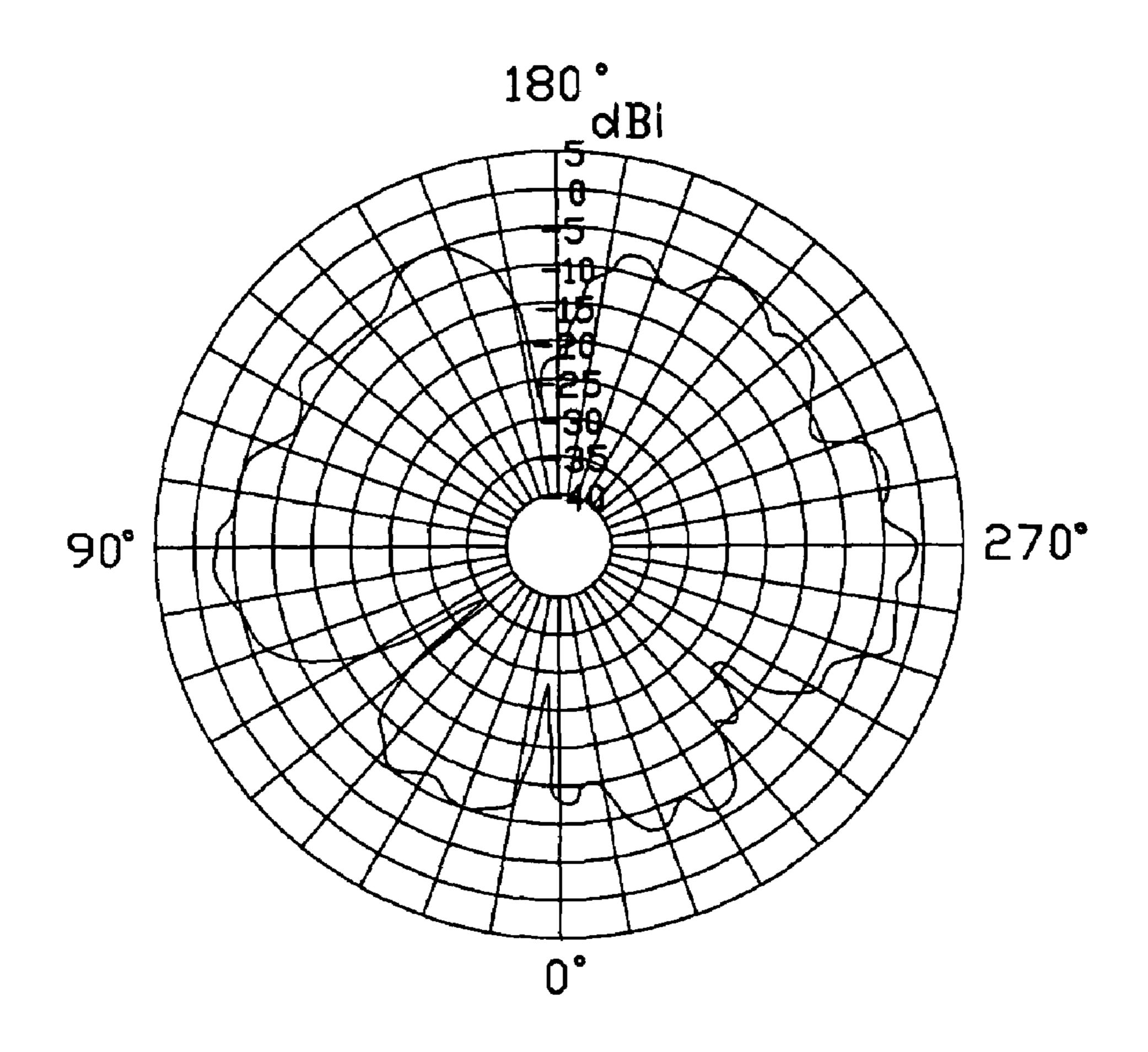
Socale: 5dBi/div Operating Frequency: 2.5GHz Horizontally polarized in X-Y plane
