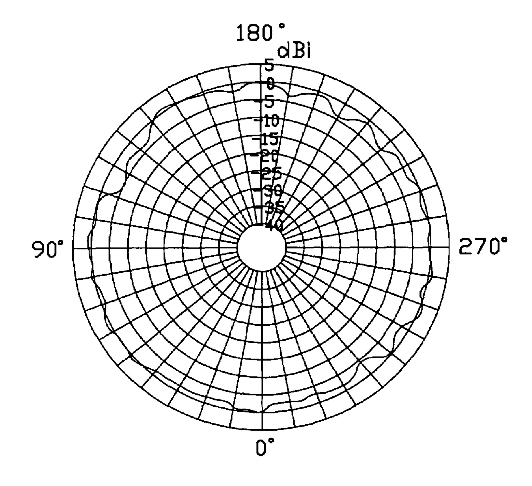
Socale: 5dBI/div Operating Frequency: 2.5GHz Vertically polarized in X-Y plane
