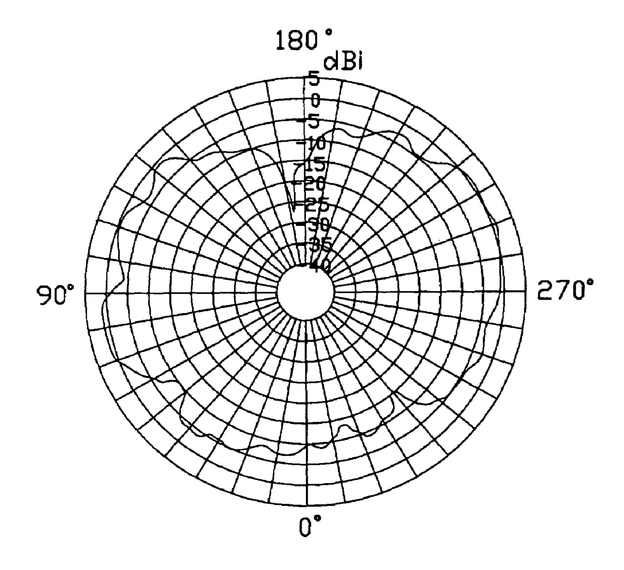
Socale: 5dBi/div Operating Frequency: 2.5GHz Horizontally polarized in Y-Z plane
