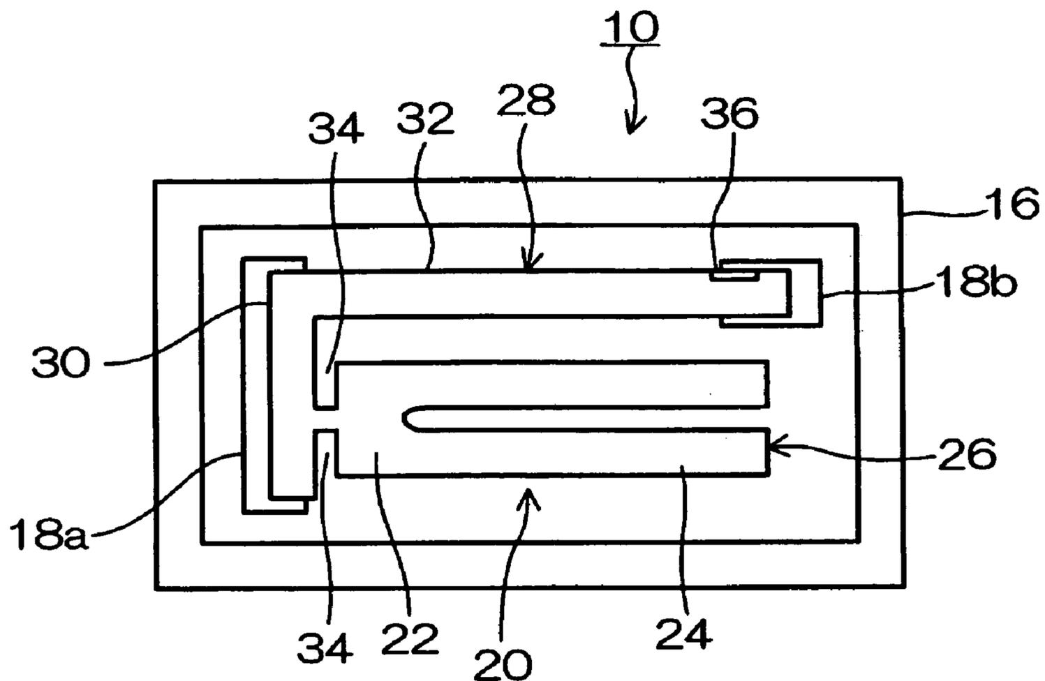
10: TUNING-FORK-TYPE PIEZOELECTRIC VIBRATOR
