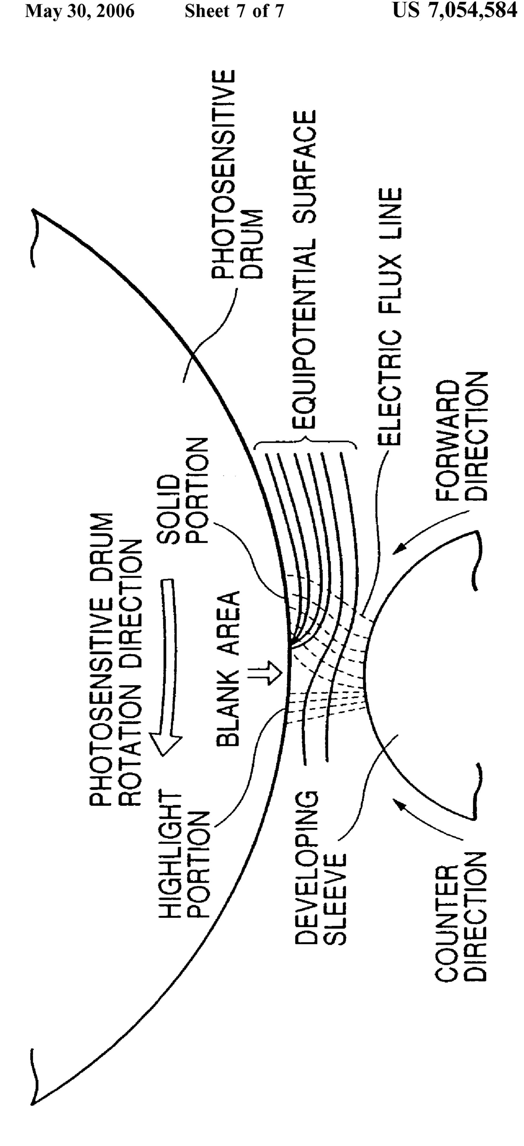
DEVELOPING APPARATUS WITH FIRST AND SECOND DEVELOPING BEARING MEMBERS EACH INCLUDING A MAGNETIC FIELD GENERATOR WHEREIN A PEAK POSITION MAGNETIC FORCE OF THE SECOND DEVELOPING MEMBERS IS A DEFINED VALUE
