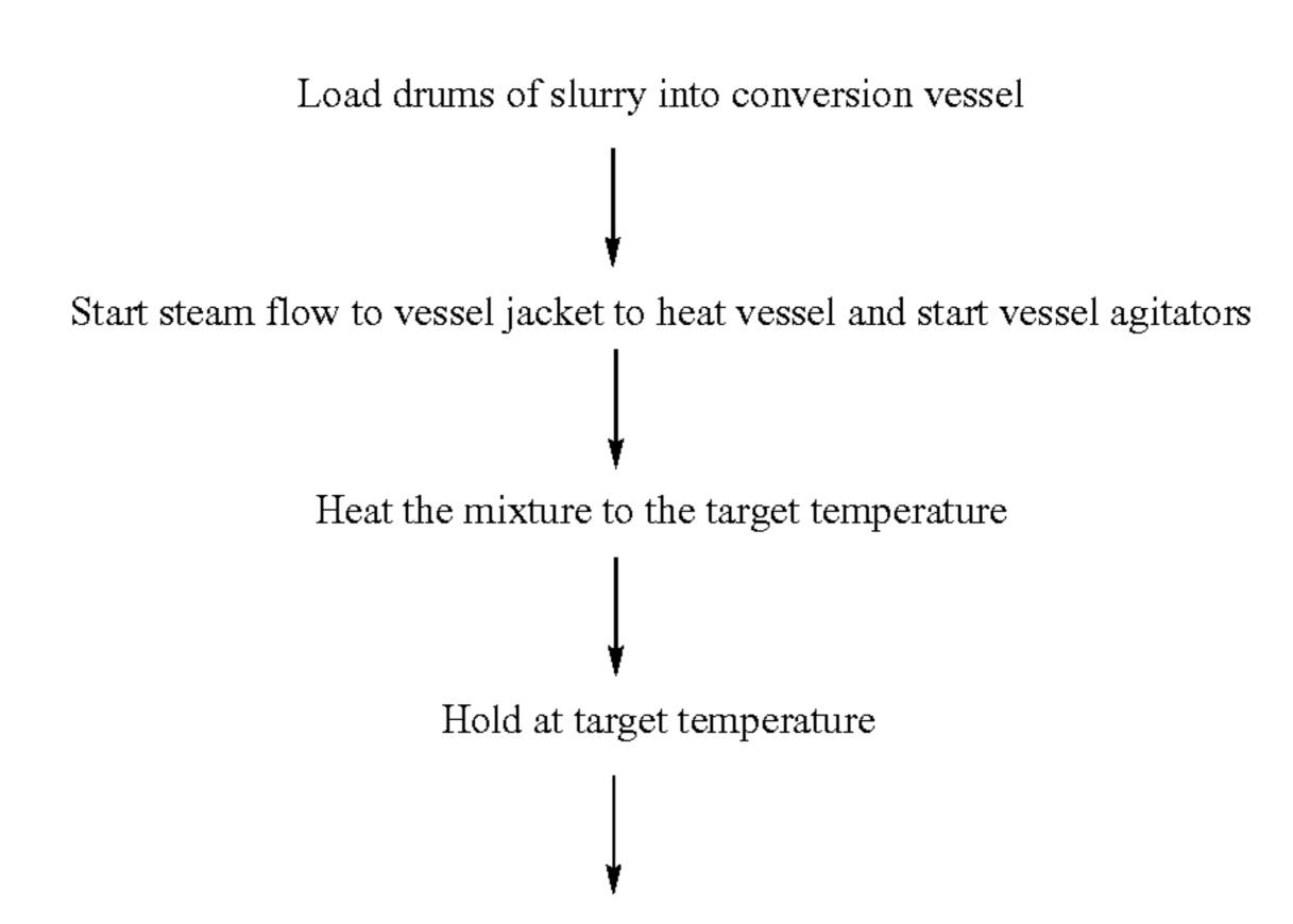
Pump resultant product to paper making machine or to spin flash drier
