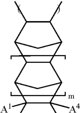
wherein  $A^1$  to  $A^4$  each independently represents a hydrogen atom, a halogen atom, a hydrocarbon group having 1–10 65 carbon atoms or a halogenated hydrocarbon group having 1–10 carbon atoms; and m is 0 or 1,
