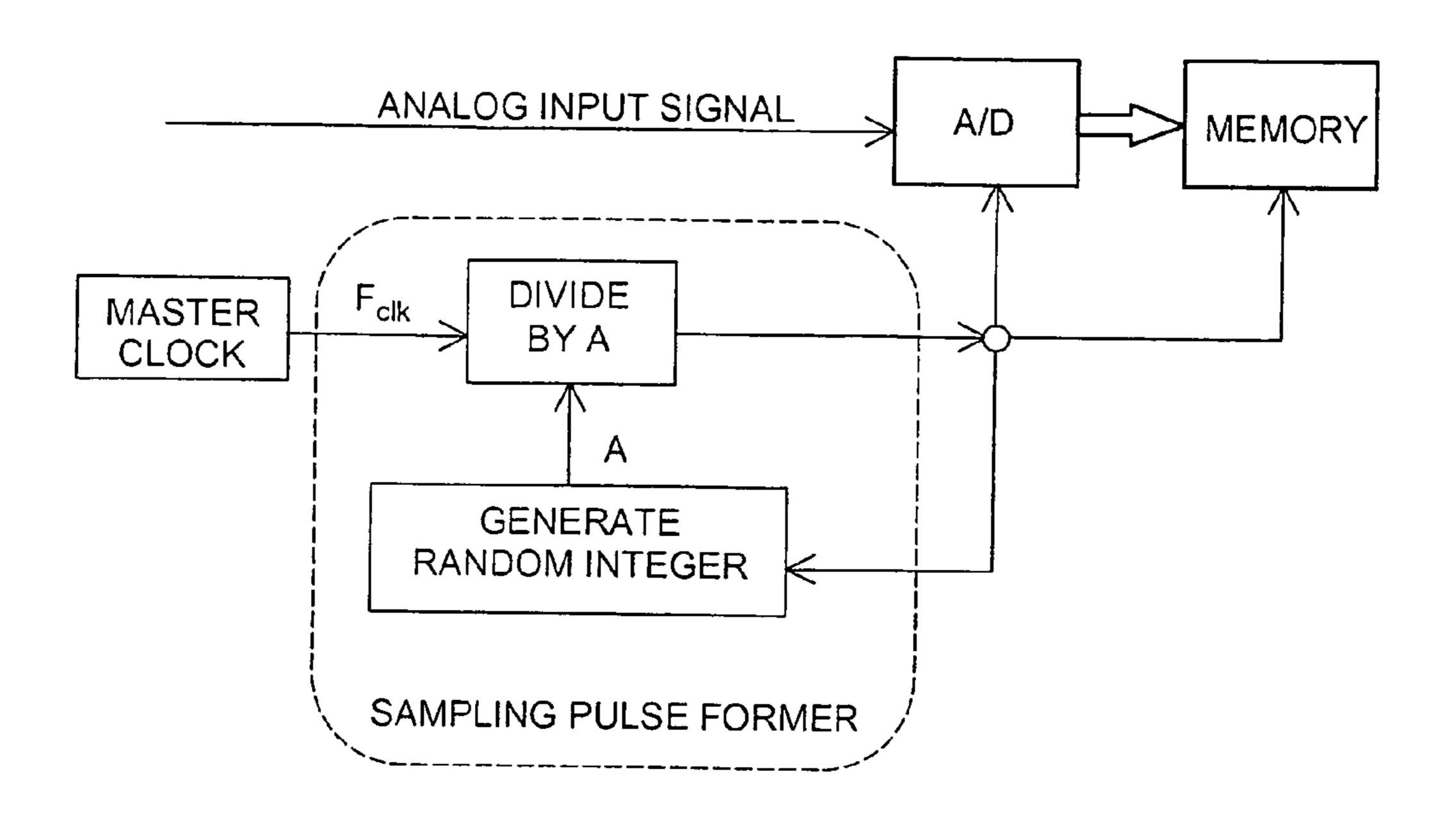
FIG. 2. A schematic block diagram of a priori art circuit
