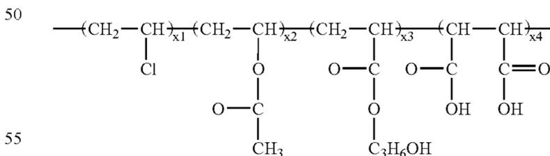
wherein x<sub>1</sub>, x<sub>2</sub>, x<sub>3</sub> and x<sub>4</sub> represent the molar percentage of each component in the polymer, and wherein the sum of x<sub>1</sub>, x<sub>2</sub>, x<sub>3</sub> and x<sub>4</sub> is equal to about 1.
