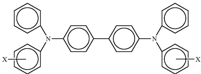
wherein X is a methyl group attached to the meta position, the weight percent illustrated herein (based on total solids) polycarbonate resin MAKROLON® 5705, a poly(4,4'-isopropylidene-diphenylene)carbonate available from Farbricken Bayer A.G., the weight percent illustrated herein of the antioxidant IRGANOX 1010®, pentaerythritol tetrakis(3-(3,5-di-tert-butyl-4-hydroxyphenyl)propionate)
