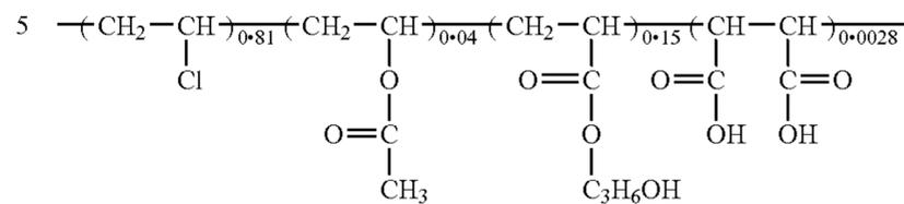
available from Union Carbide, applied as a solution in methylene chloride 17 weight percent. The coated devices were heated in an oven maintained at from about 40° C. to about 100° C. for over 30 minutes to form a charge transport layer having a thickness of 25 micrometers.
