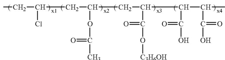
wherein  $x_1$ ,  $x_2$ ,  $x_3$  and  $x_4$  represent the molar percentage of each component in the polymer, and wherein the sum of  $x_1$ ,  $x_2$ ,  $x_3$  and  $x_4$  is equal to 1.
