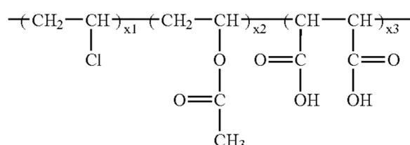
wherein  $x_1$ ,  $x_2$ , and  $x_3$  represent the molar percentage of each component in the polymer, and the sum of  $x_1$ ,  $x_2$ , and  $x_3$  is equal to 1.
