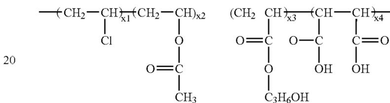
wherein x<sub>1</sub>, x<sub>2</sub>, x<sub>3</sub> and x<sub>4</sub> represent the molar percentage of each component in the polymer, and wherein the sum of x<sub>1</sub>, x<sub>2</sub>, x<sub>3</sub> and x<sub>4</sub> is equal to 1.
