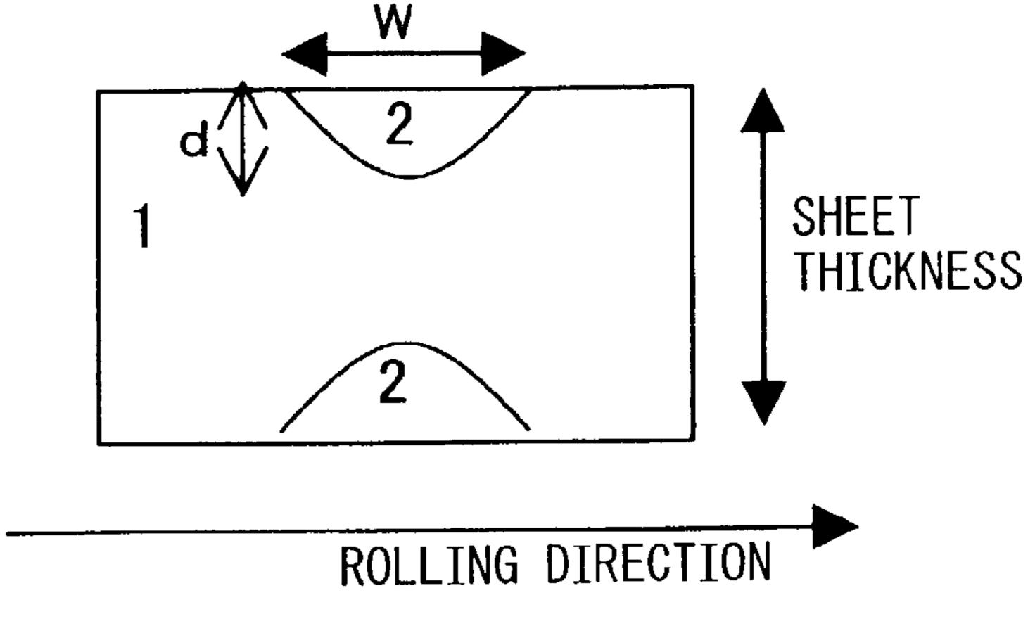
ASPECT RATIO OF MELTED AND RE-SOLIDIFIED LAYER=d/W
