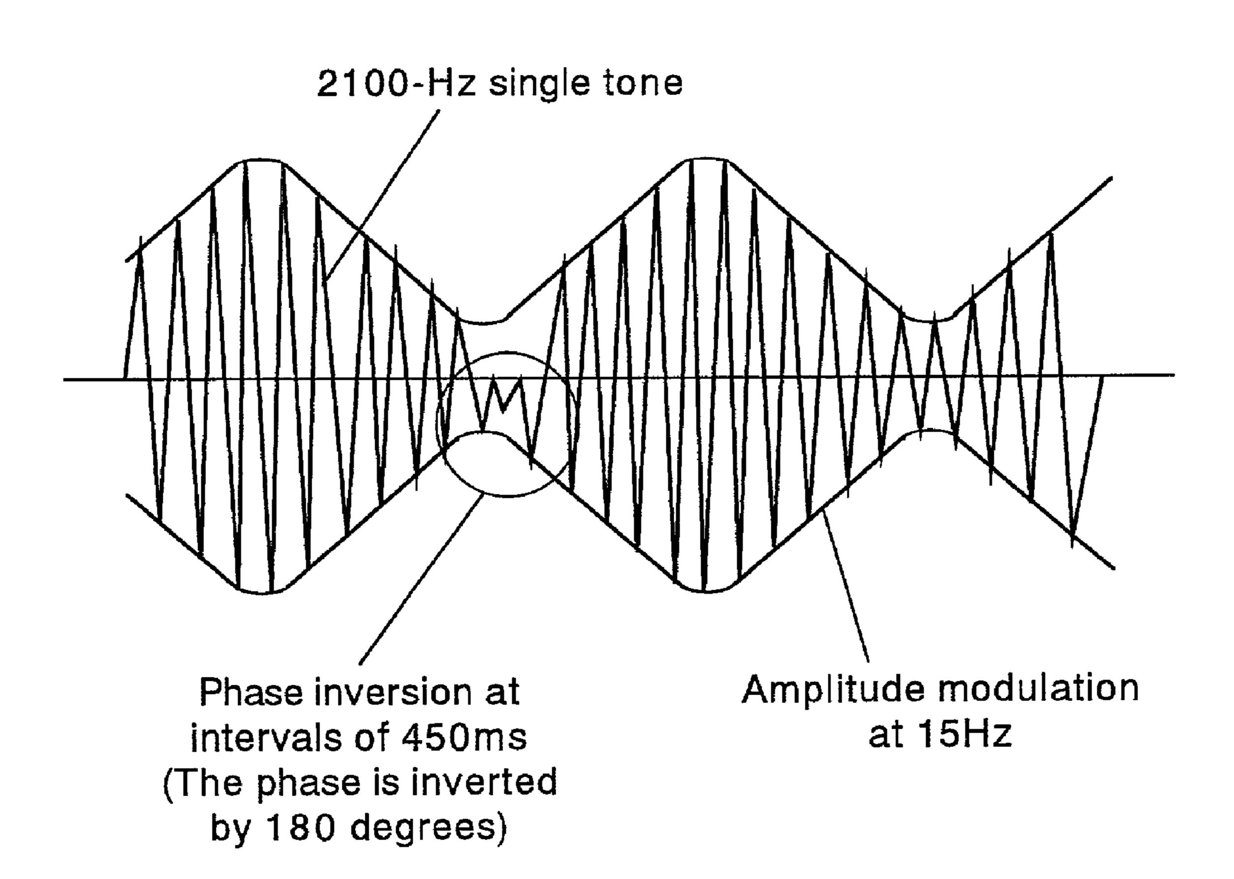
Input signal from a telephone, a fax machine or a terminal
