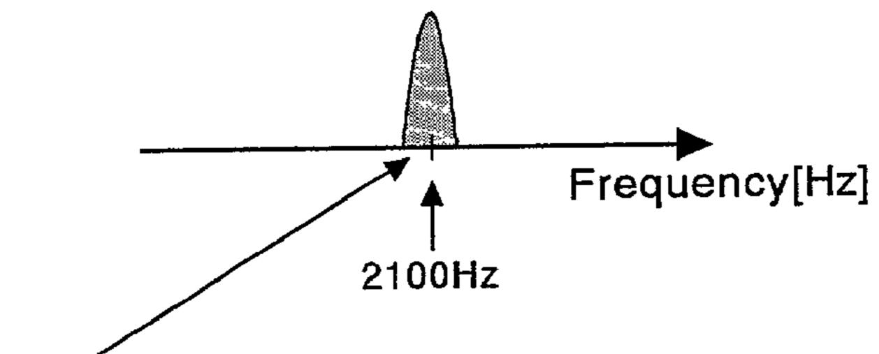
A newly created 2100Hz component (2100Hz single tone) is inserted. The 2100Hz single tone does not include ±15Hz components (or is not amplitude-modulated at 15Hz)
