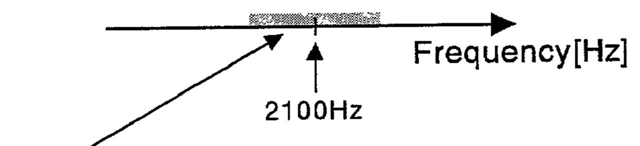
The filter removes components of 2,100  $\pm$  15Hz At that time, the 2100Hz component and components of  $\pm$  15Hz relative to 2100Hz are removed.
