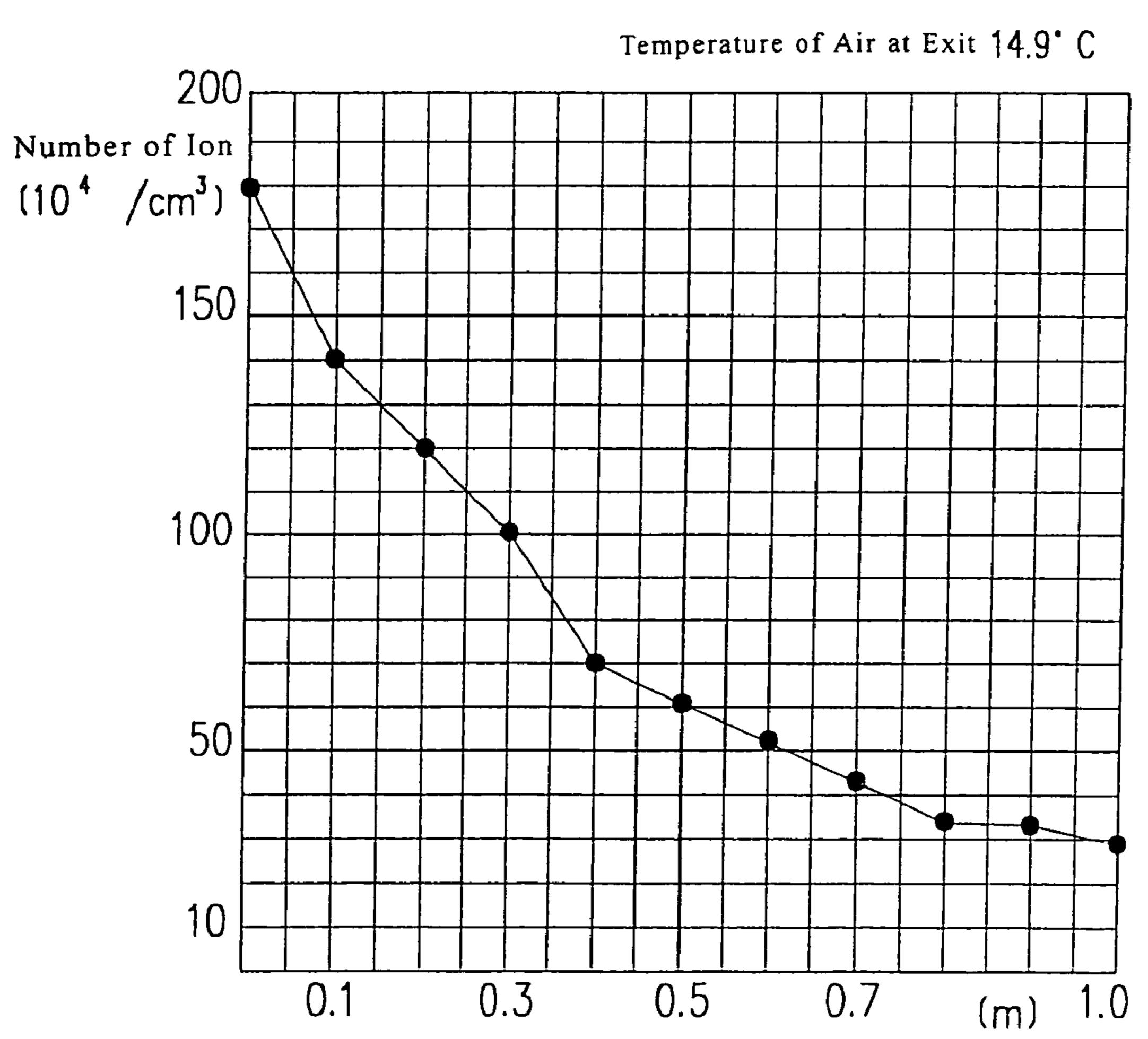
Distance Measured from Minus Ion Generation Apparatus
