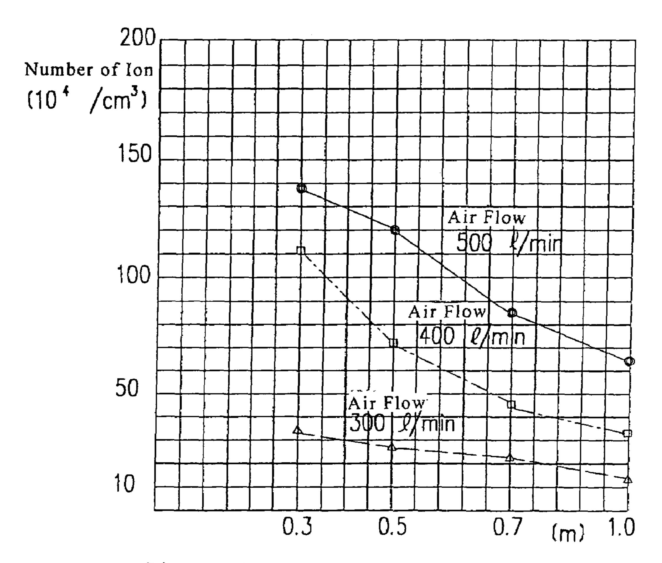
Distance Measured from Minus Ion Generation Apparatus
