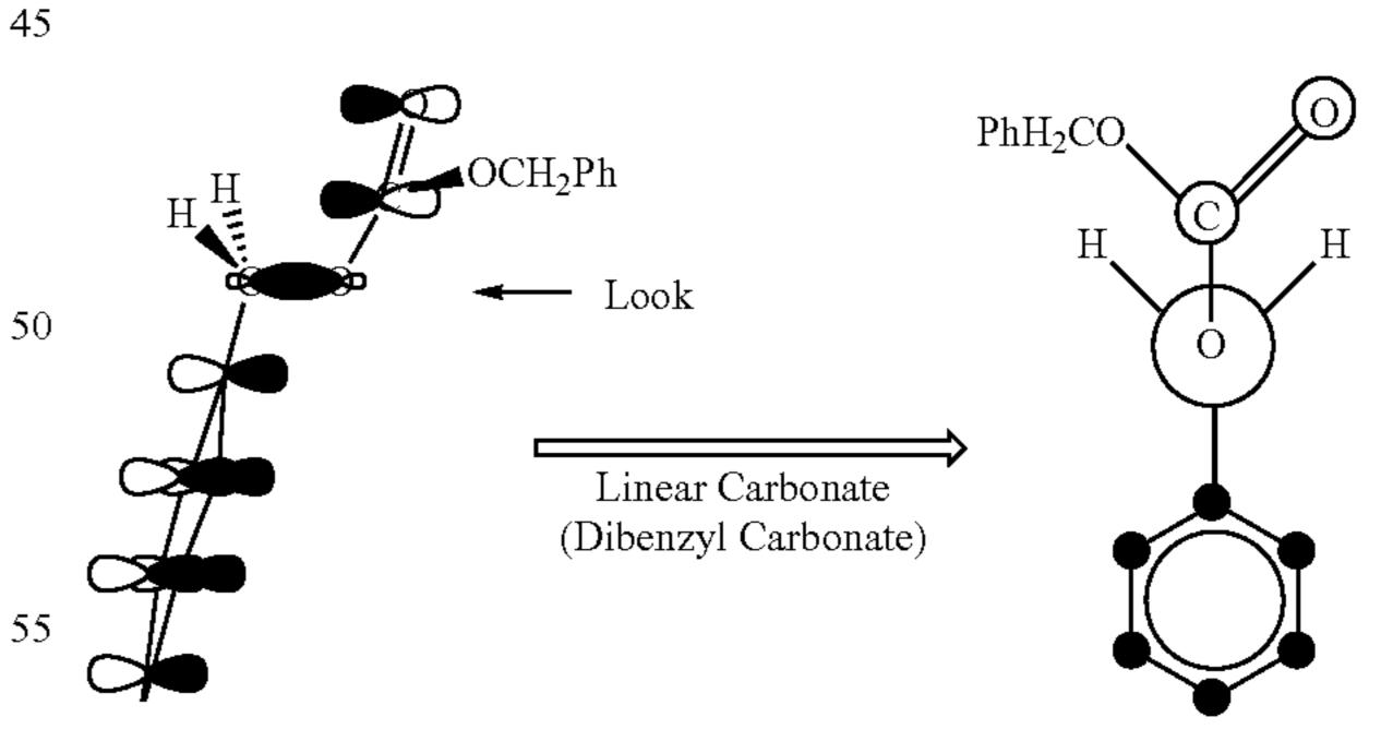
The flexibility of this linear carbonate makes it possible for the molecule to adopt the right conformation for easy bond cleavage. In that manner, the existence of orbital interaction lowers the activation energy for C—O bond cleavage in the anion radical intermediate.
