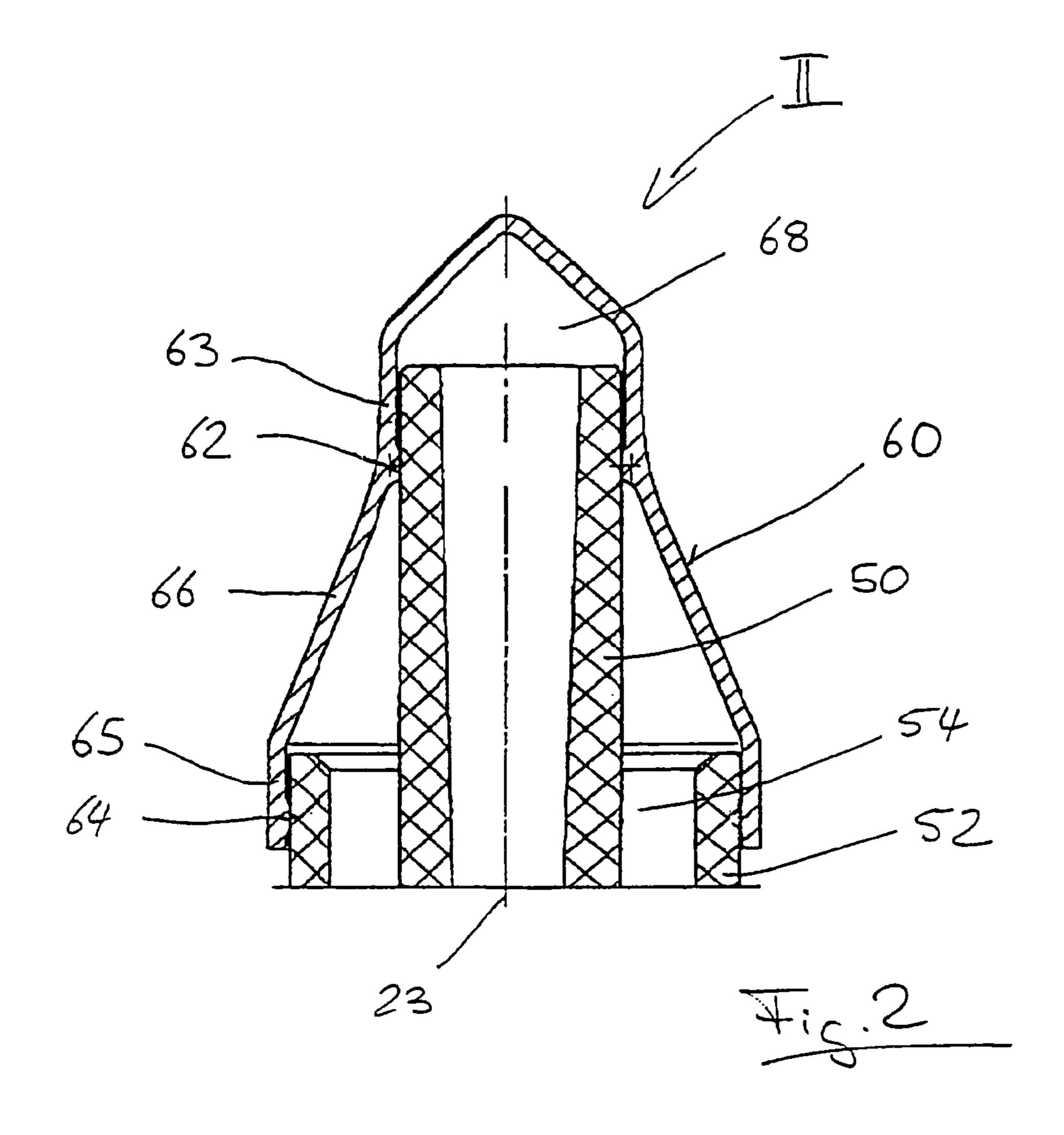
The invention relates to an apparatus for the sealing of inflatable articles, in particular tyres, comprising a container containing a sealant and an extraction unit releasably connected and preferably screwed to the container, the removal unit having at least one inlet line connectable to a source of gas pressure and at least one outlet line capable of being coupled to the article to be sealed.
