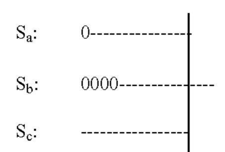
With reference to FIG. 3, input 303 to fixed point gen- 25 erator 245 contains the shifted and truncated masks of  $S_a$ ,  $S_b$ as shown above. In addition, input 305 is a carries mask  $M_C$ ="0xx . . . xC<sub>p</sub>", where  $C_p \in \{0, 1, 2\}$  has the contribution of the tails, which combines the effects of carry and of rounding.
