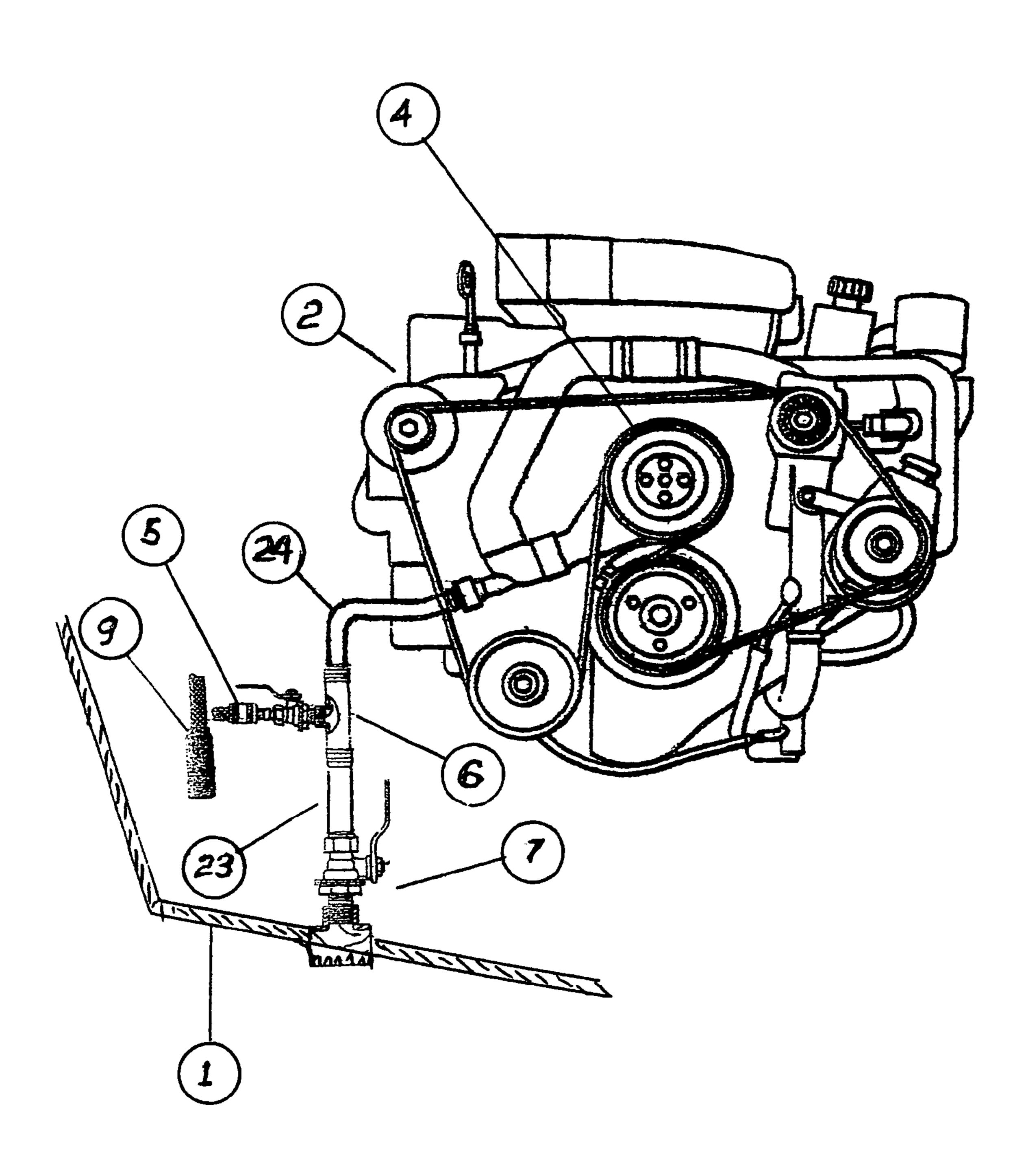
QUICKFLUSH VALVE KIT FOR FLUSHING AND WINTERIZING OF COOLING SYSTEM OF INBOARD MARINE ENGINES, POWER GENERATORS, AIR-CONDITIONING UNITS, AND SAILBOAT ENGINES
