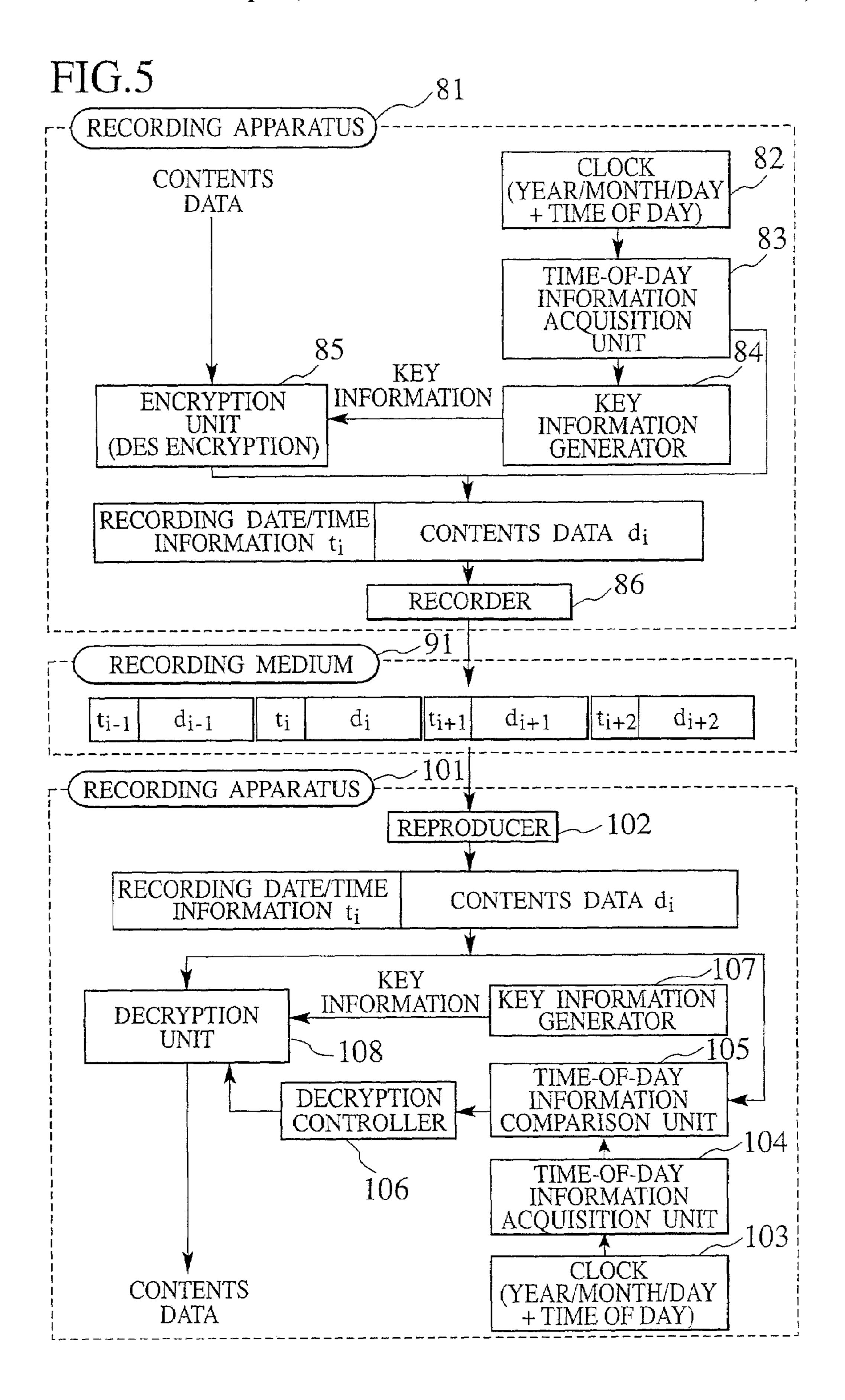
CONTENTS RECORDING APPARATUS, RECORDING MEDIUM, CONTENTS REPRODUCING APPARATUS, CONTENTS TRANSMISSION METHOD, TRANSMISSION MEDIUM, AND CONTENTS RECEPTION METHOD
