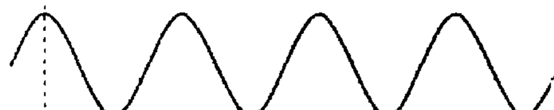
FIG. 16C DRIVE CURRENT OF THIRD SENSOR PROBE
