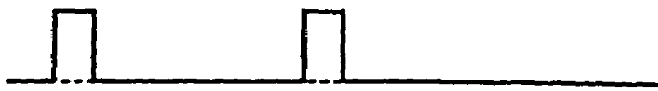
FIG. 18C OUTPUT SIGNAL OF COMPARATOR
