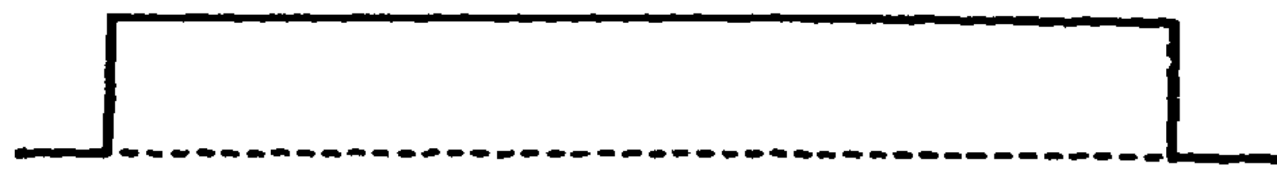
FIG. 18D OUTPUT SIGNAL OF RE-TRIGGERABLE FF CIRCUIT
