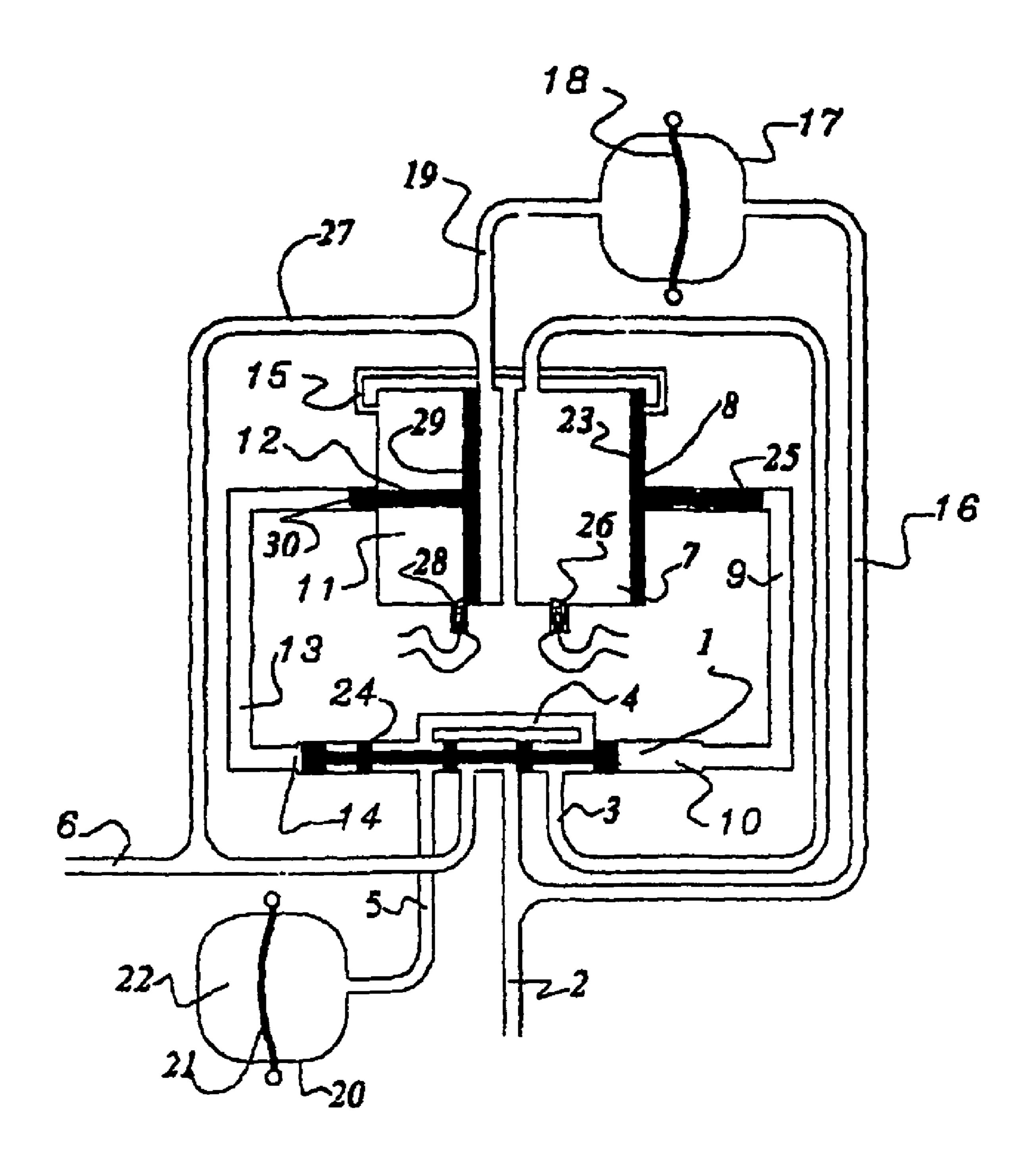
This invention relates to a valve for use in controlling the flow of a transmitted fluid and in particular to a valve that is actuated between open and closed positions using the pres- 5
