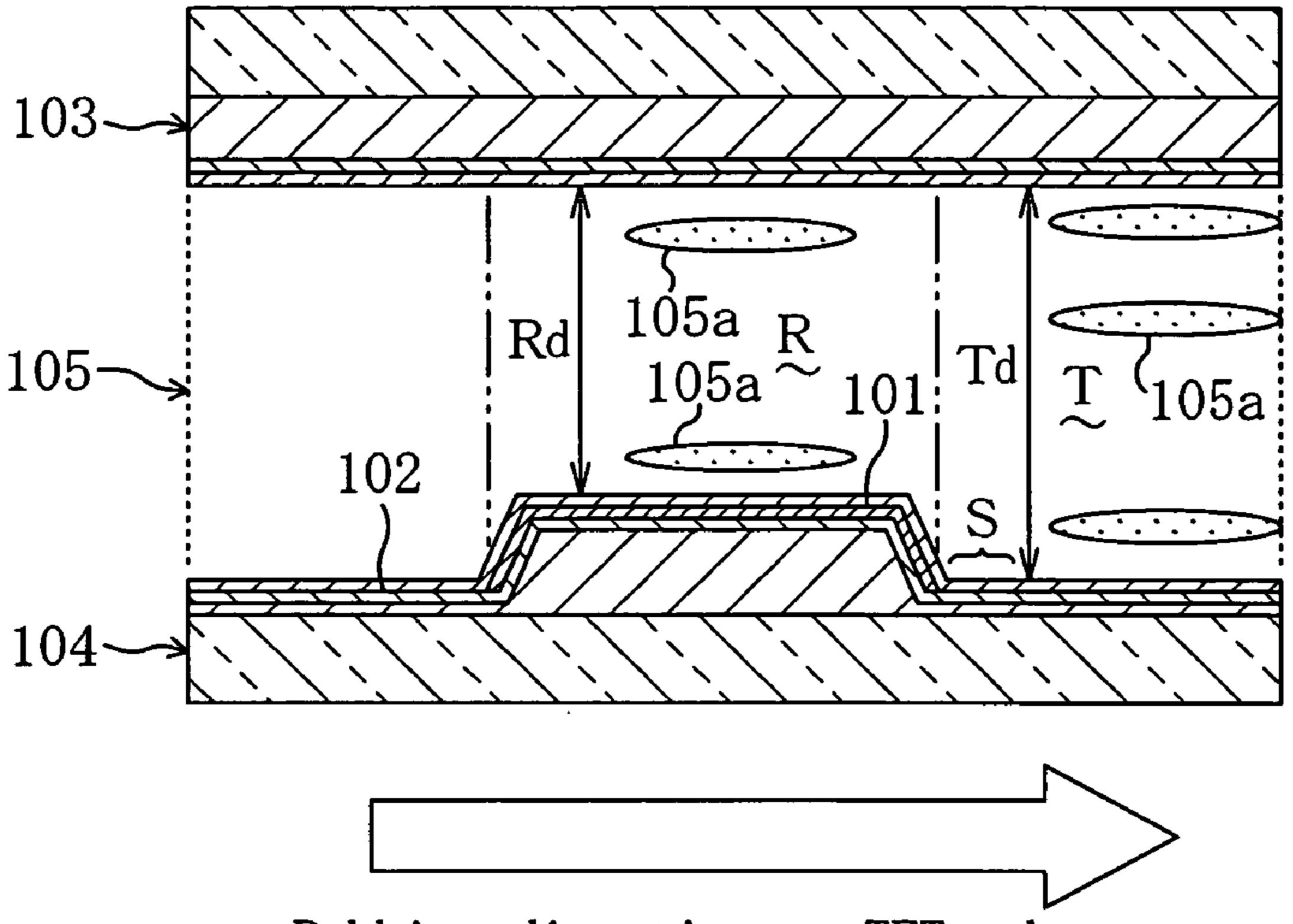
Rubbing direction on TFT substrate
