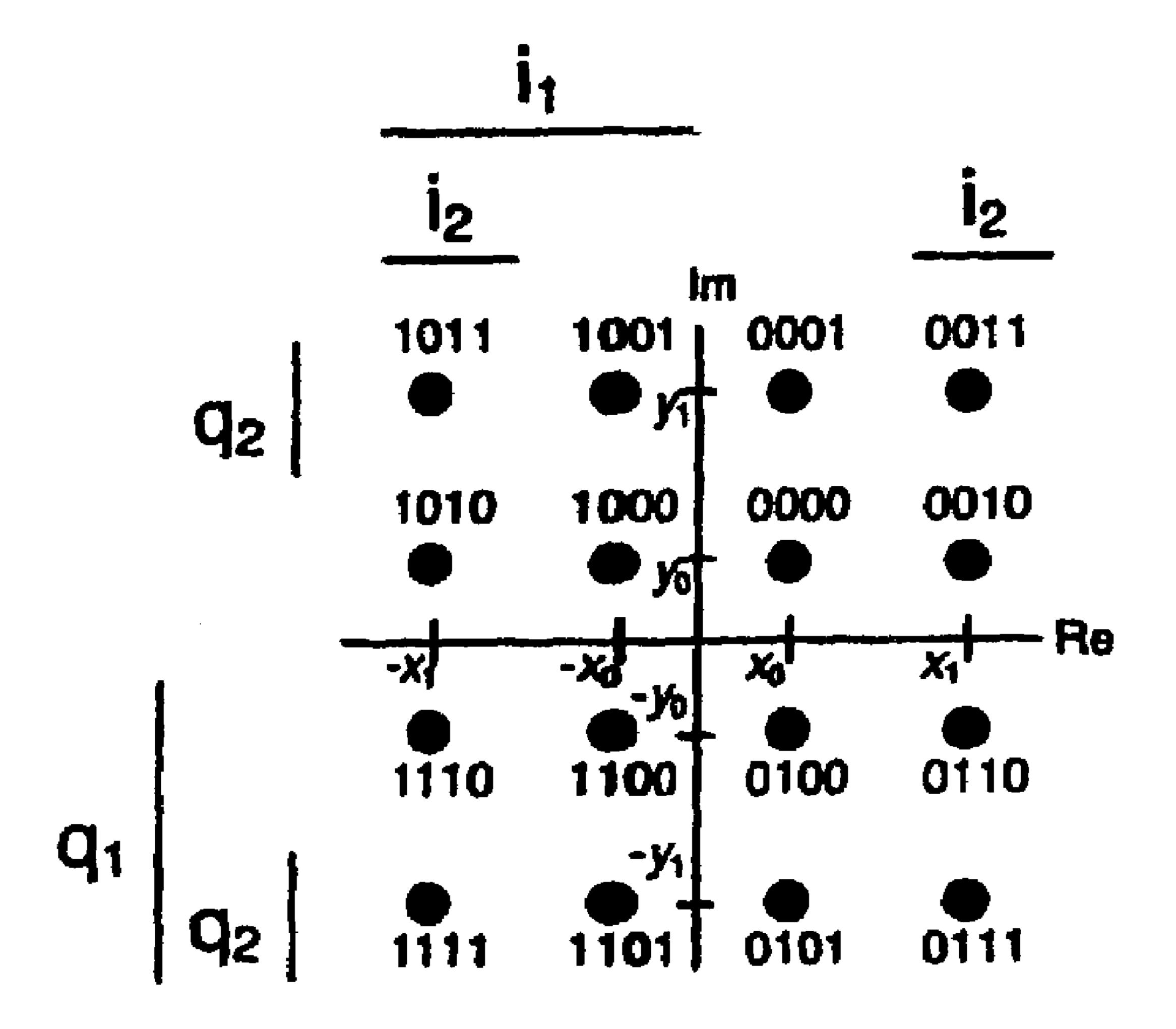
bit-mapping order: i<sub>1</sub> q<sub>1</sub> i<sub>2</sub> q<sub>2</sub> MSBs: i<sub>1</sub> q<sub>1</sub> LSBs: i<sub>2</sub> q<sub>2</sub>
