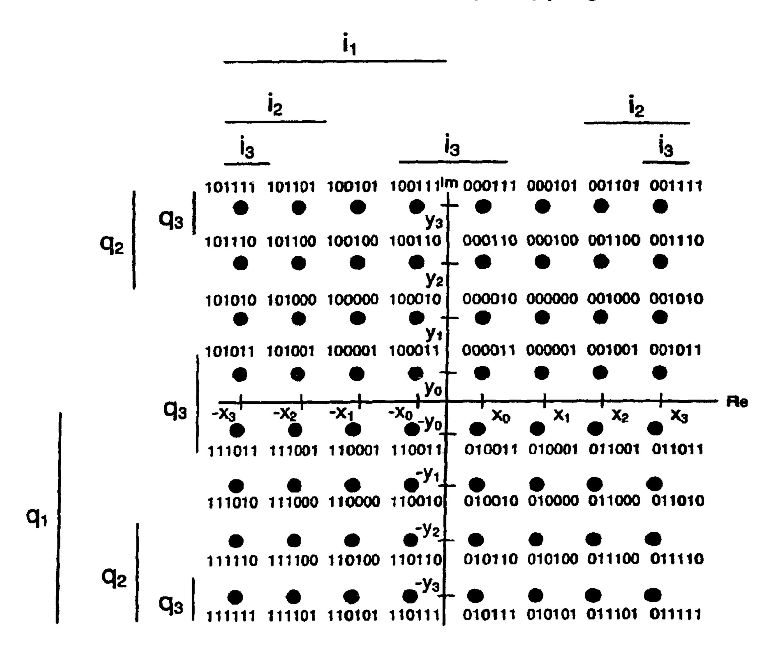
bit-mapping order: i<sub>1</sub> q<sub>1</sub> i<sub>2</sub> q<sub>2</sub> i<sub>3</sub> q<sub>3</sub>
