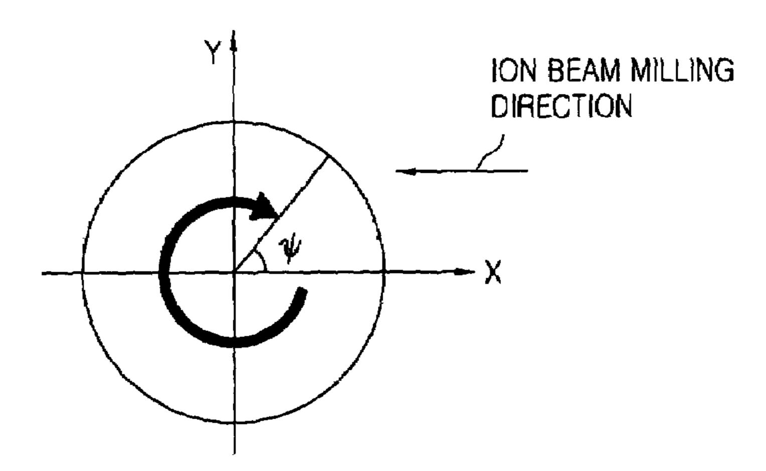
TANGENTIAL SURFACE DIRECTION:  $(x,y,z)=(-\sin\theta\cos\psi,-\sin\theta\sin\psi,\cos\theta)$ MILLING DIRECTION:  $(x,y,z)=(\cos\Phi,0,\sin\Phi)$
