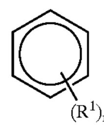
wherein n is an integer from 0 to about 3, and wherein each  $R^1$  is independently selected from the group consisting of 10 hydrogen and  $C_{1-5}$  alkyl moieties, with the balance of the 6-n bonds being to hydrogen.
