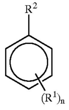
wherein n is an integer from 0 to about 3; each  $R^1$  is independently selected from the group consisting of hydrogen and  $C_{1-5}$  alkyl moieties; and  $R^2$  is selected from  $C_{2-5}$  alkyl moieties, with the balance of the 5-n bonds being to hydrogen. More preferred  $C_{2-5}$  alkyl-substituted aromatic compounds consistent with the aforementioned formula include ethylbenzene, ethyltoluene, isopropylbenzene,
