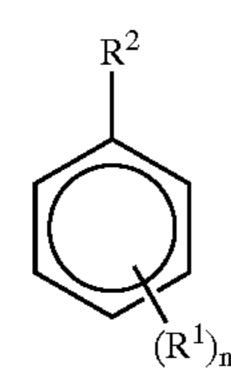
wherein n is an integer from 0 to about 3; each  $R^1$  is independently selected from the group consisting of hydrogen and  $C_{1-5}$  alkyl moieties; and  $R^2$  is a  $C_{2-5}$  alkyl moiety, with the balance of the 5-n bonds being to hydrogen.
