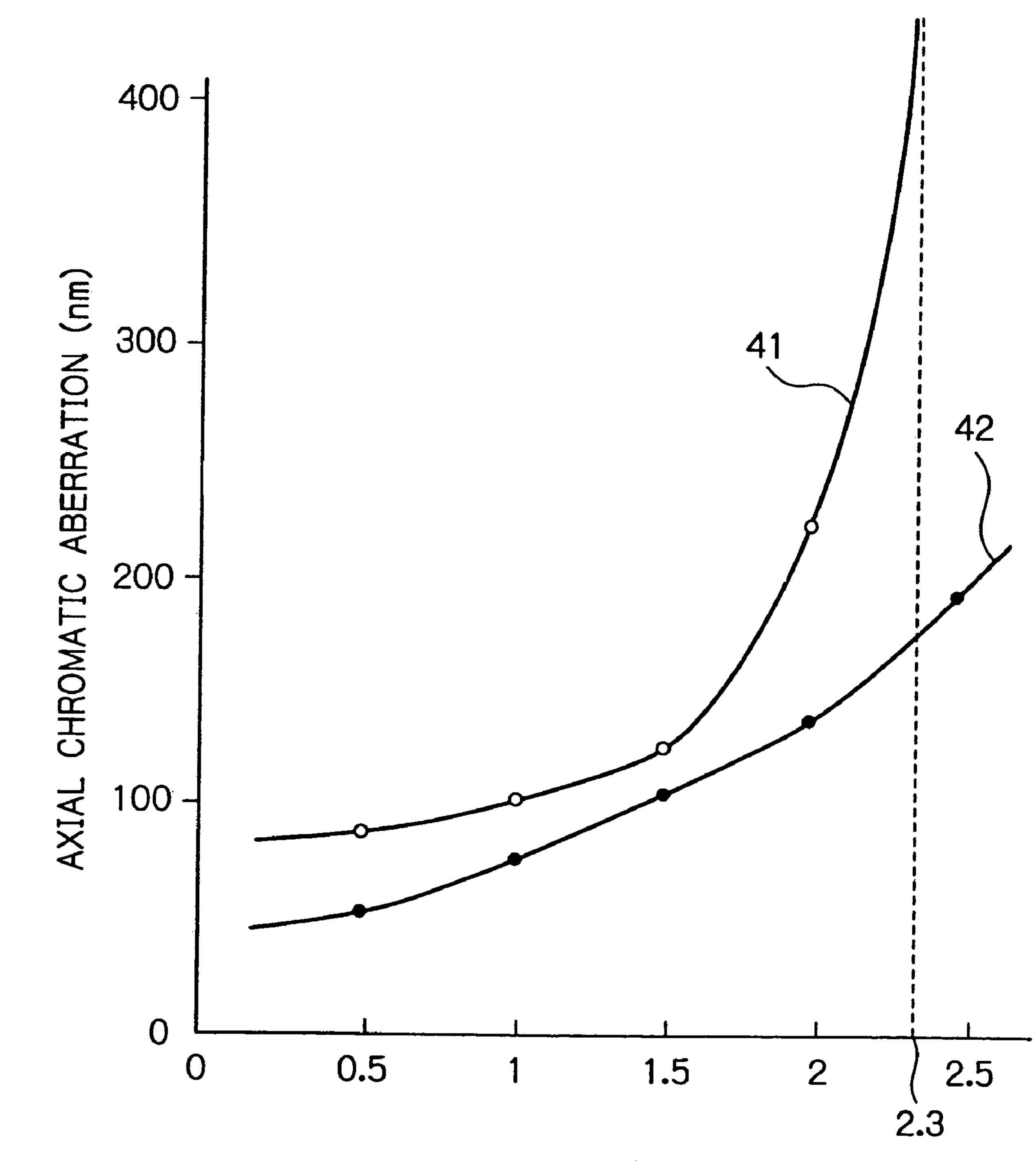
THICKNESS OF CENTRAL ELECTRODE 19 (mm)
