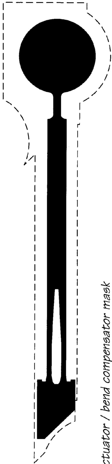
Actuator / bend compensator mask
