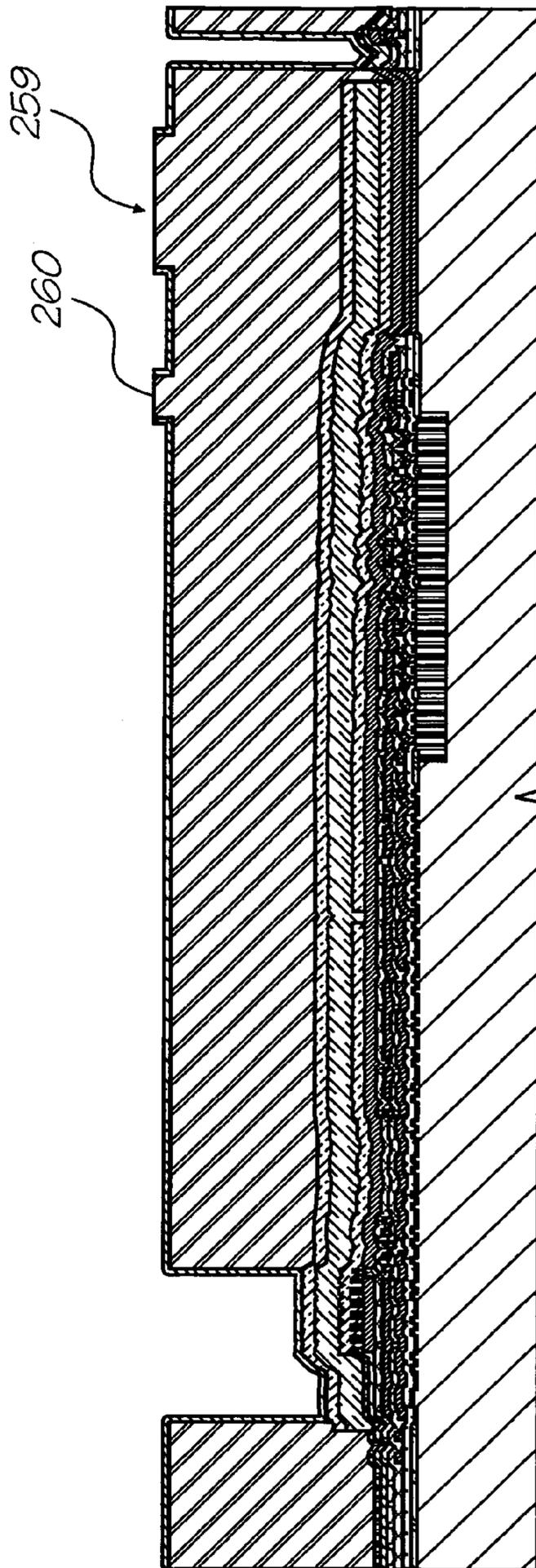
Form self-aligned nozzles using CMP
