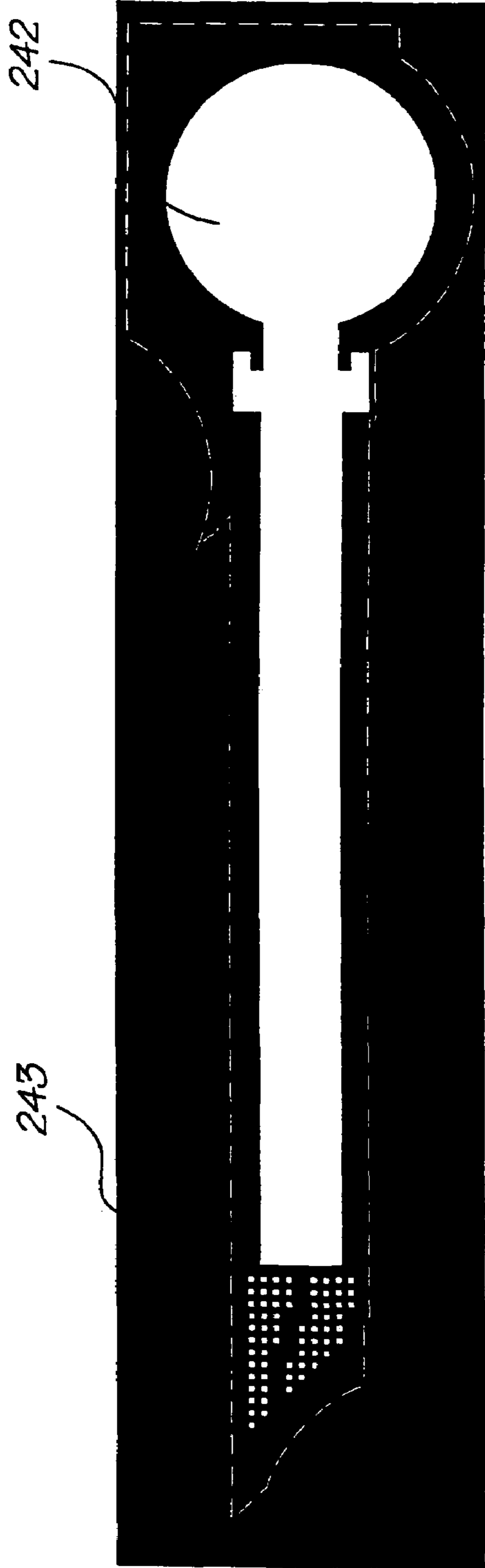
Via 3 / Passivation mask
