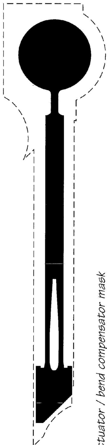
Actuator / bend compensator mask
