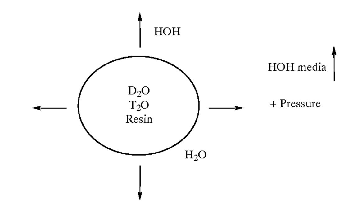
During periods of cyclic lower pressure within the slurry, the hydration sites vacated by the  $H_2O$  squeezed from the resin are filled with  $D_2O$  and  $T_2O$  as shown herebelow.
