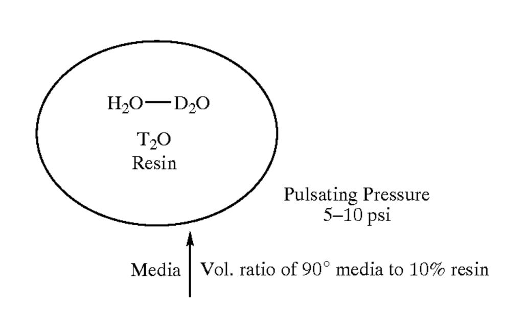
During periods of higher pressure within the flowing slurry, in HOH is squeezed from the resin while DOD and TOT are forced into the resin on a molecular exchange basis as shown herebelow:
