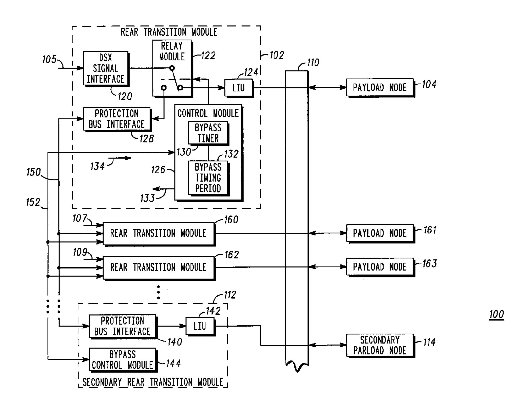
100 SECONDARY Parload node NODE NODE NODE PAYLOAD PAYLOAD **PAYLOAD** MODULE 162 160 TRANSITION MODULE BYPASS TIMER BYPASS TIMING PERIOD MODULE 4 CONTROL MODULE MODULE 130 TRANSITION RELAY MODULE TRANSITION **TRANSITION** 126 BYPASS CONTROL MODULE INTERFACE PROTECTION BUS INTERFACE REAR PROTECTION REAR REAR REAR SIGNAL INTERFACE SECONDARY 134 107 109
