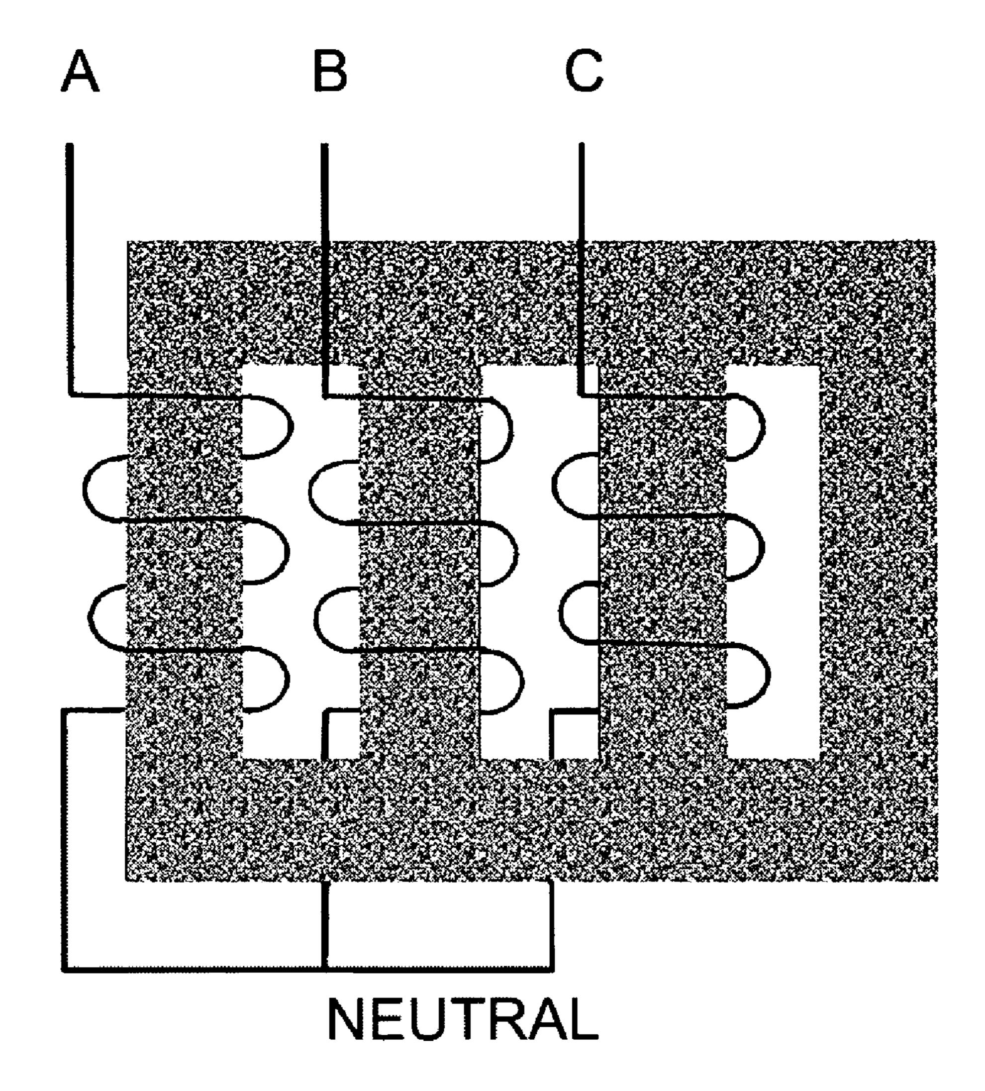
THREE-PHASE, 4-LIMB CONSTRUCTION TO GIVE HIGH ZERO-SEQUENCE IMPEDANCE
