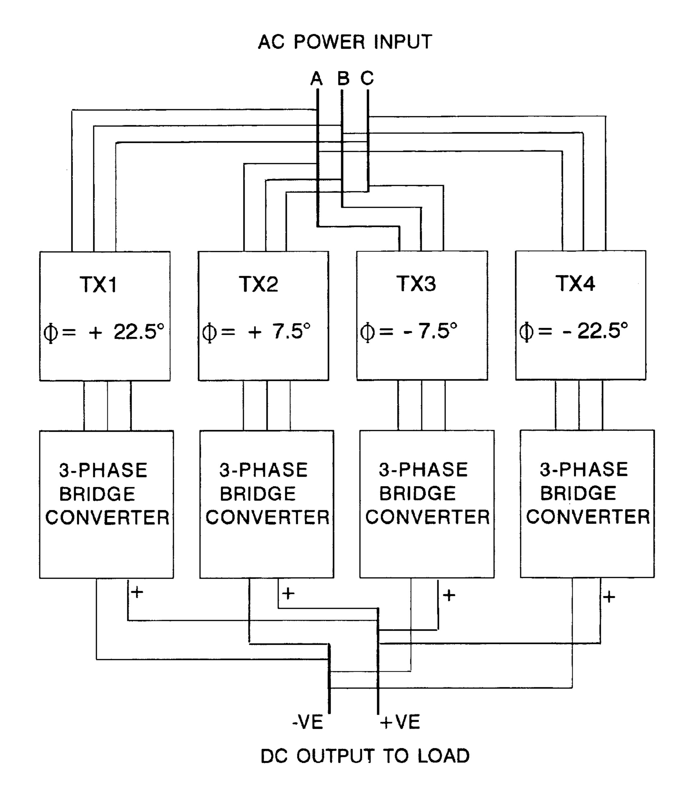
TX1,TX2,TX3, AND TX4 ARE HIGH ZERO-SEQUENCE IMPEDANCE 1:1 AUTOTRANSFORMERS WITH ISOLATED NEUTRAL AND PHASE SHIFT AS INDICATED.
