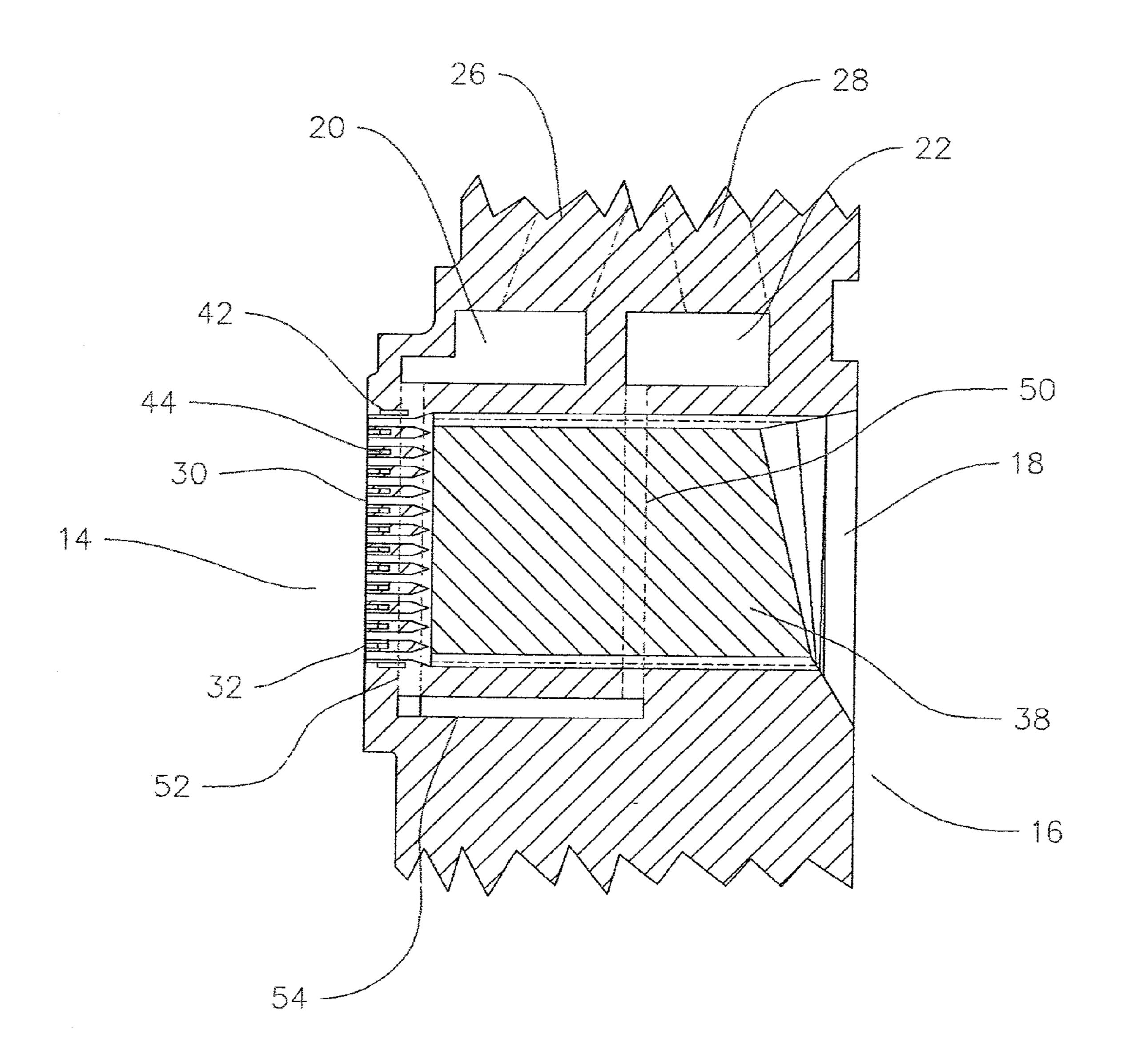
PELLETIZING DIE WITH EVEN HEAT DISTRIBUTION AND WITH POLYMER CHANNEL TO ORIFICE TRANSITION ZONE, PROCESS FOR ORIFICE THERMAL STABILIZATION AND PROCESS FOR FORMING A PELLETIZING DIE WITH BRAZING AND THIN HARD FACE LAYER
