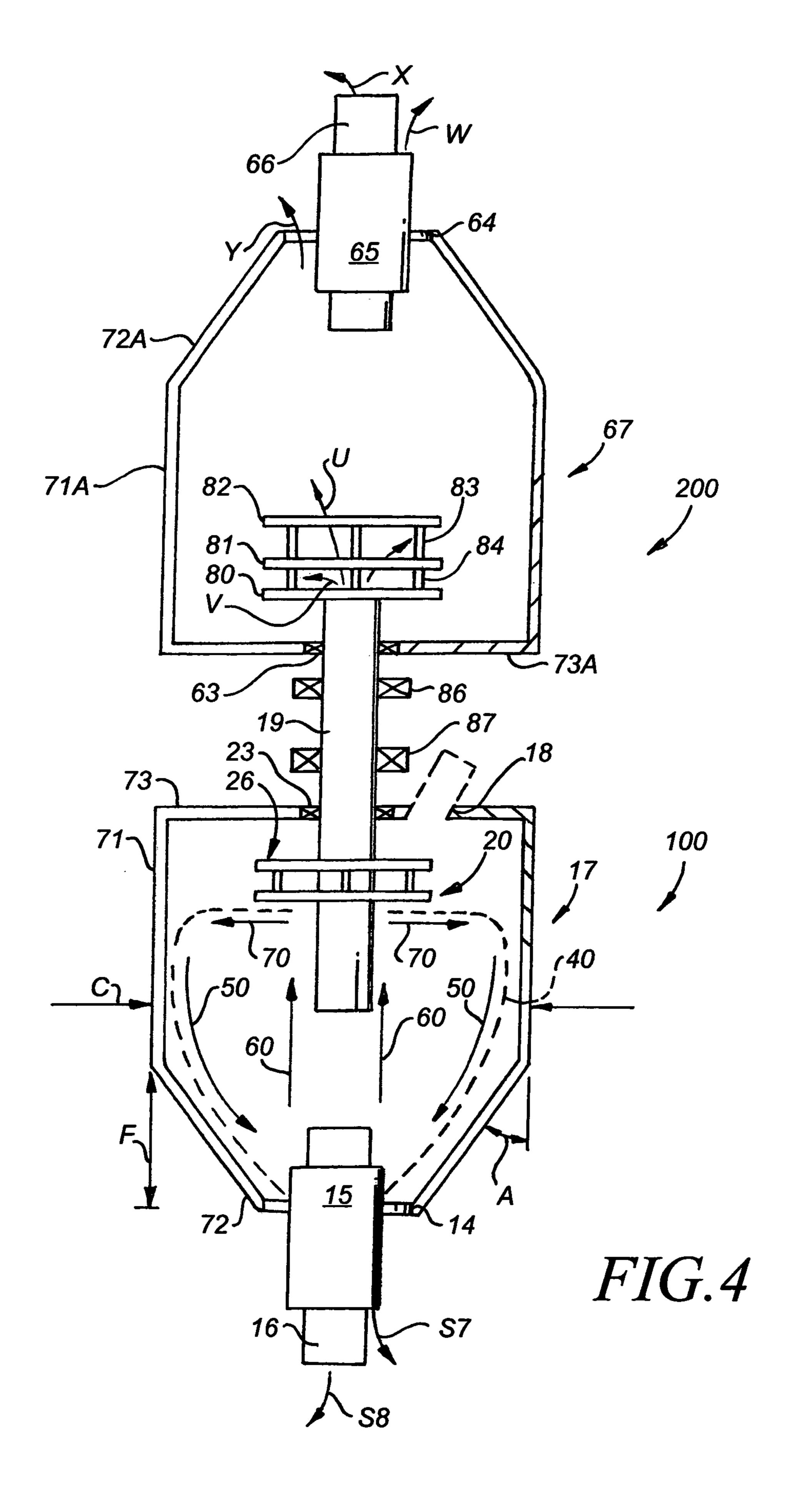
PETROLEUM DRILLING METHOD AND APPARATUS TO COOL AND CLEAN DRILL BIT WITH RECIRCULATING FLUID **COMPOSITION WHILE RECLAIMING** MOST WATER UTILIZED AND GREATLY REDUCING THE NORMAL CONSUMPTION OF WATER DURING DRILLING
